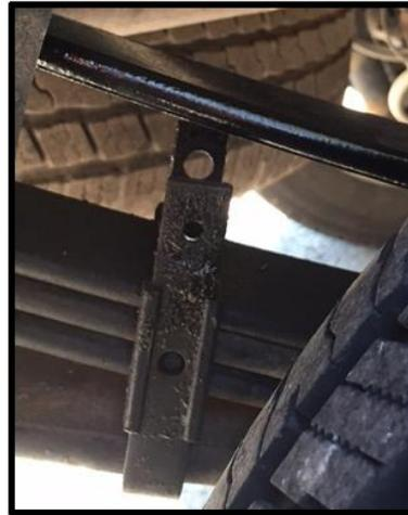
Remove rear clip bolt and roller on Titan models that are attached with a removable nut and bolt. Do not remove bracket.
