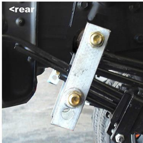
Place PSP-19 on top of spring plate flat side up facing, with groove toward the front
