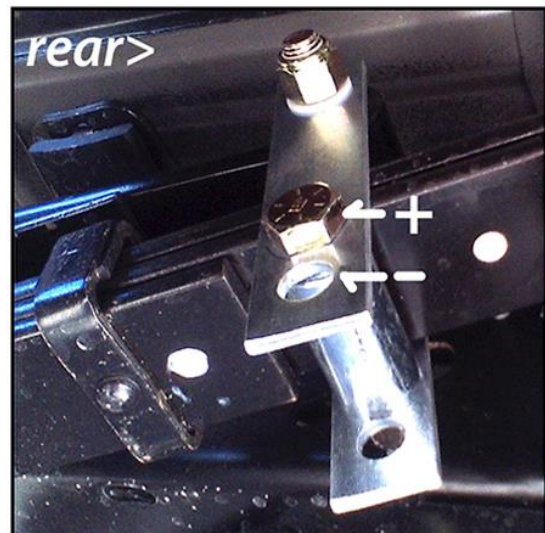
Rear Shackle installation
