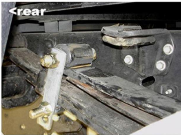
Place PSP11 on top of spring plate flat side up facing, with groove toward the front
