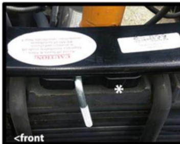
Place PSP11 on top of spring plate flat side up facing, with groove toward the front
