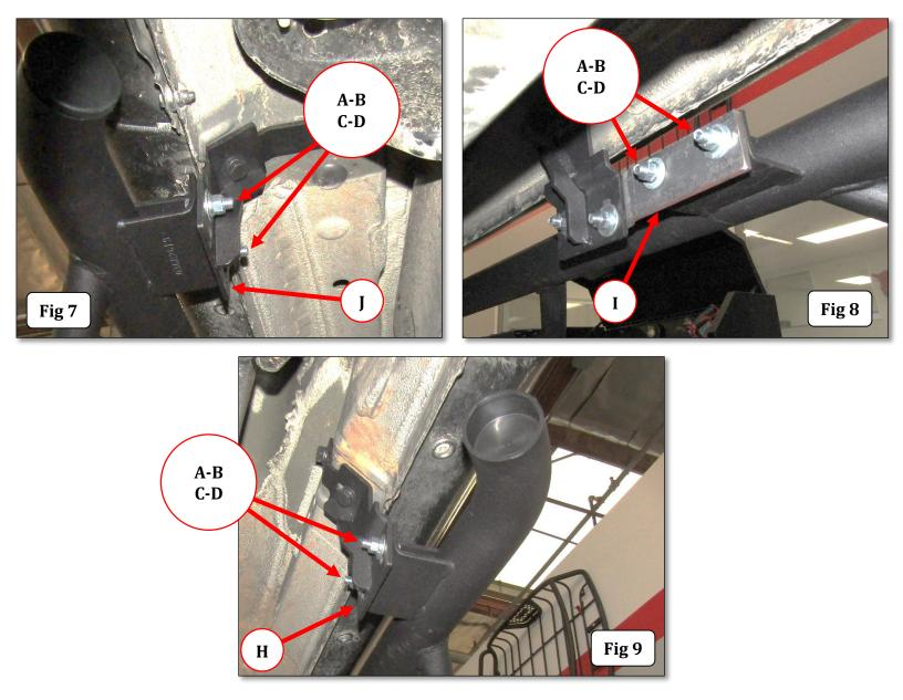
**Step-4.1 International Models:** With assistance, attach the Dominator D2 side step to the front, center and rear bracket using (2) 3/8" x 1 ¼" hex bolts, (2) 3/8" lock washers, (4) 3/8" flat washers, and (2) 3/8" hex nuts for each bracket.
