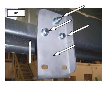
**STEP-2** ATTACH ONE OF THE MOUNTING BRACKETS TO THE BODY PANEL USING THE T-PLATE (2) 3/8" X 1 1/4" HEX BOLTS, (3) 3/8" FLAT WASHERS, (3) 3/8" LOCK WASHERS AND (1) 3/8" HEX NUT. HAND TIGHTEN. REPEAT THE ABOVE PROCEDURE TO INSTALL THE CENTER AND REAR MOUNTING BRACKETS. **PHOTO'S #2 & #3**
