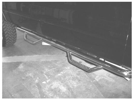
STEP 5. Align sidestep with the body, and then tighten all mounting bracket and sidestep nuts and
