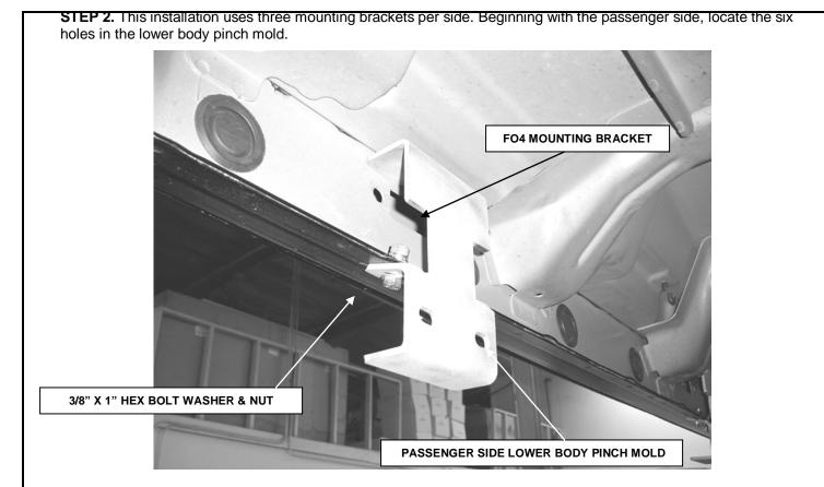
**STEP 3.** Loosely attach the flange of the mounting brackets to the bottom of the lower body pinch mold using the 3/8" x 1" hex bolts, washers, and nuts as shown.
