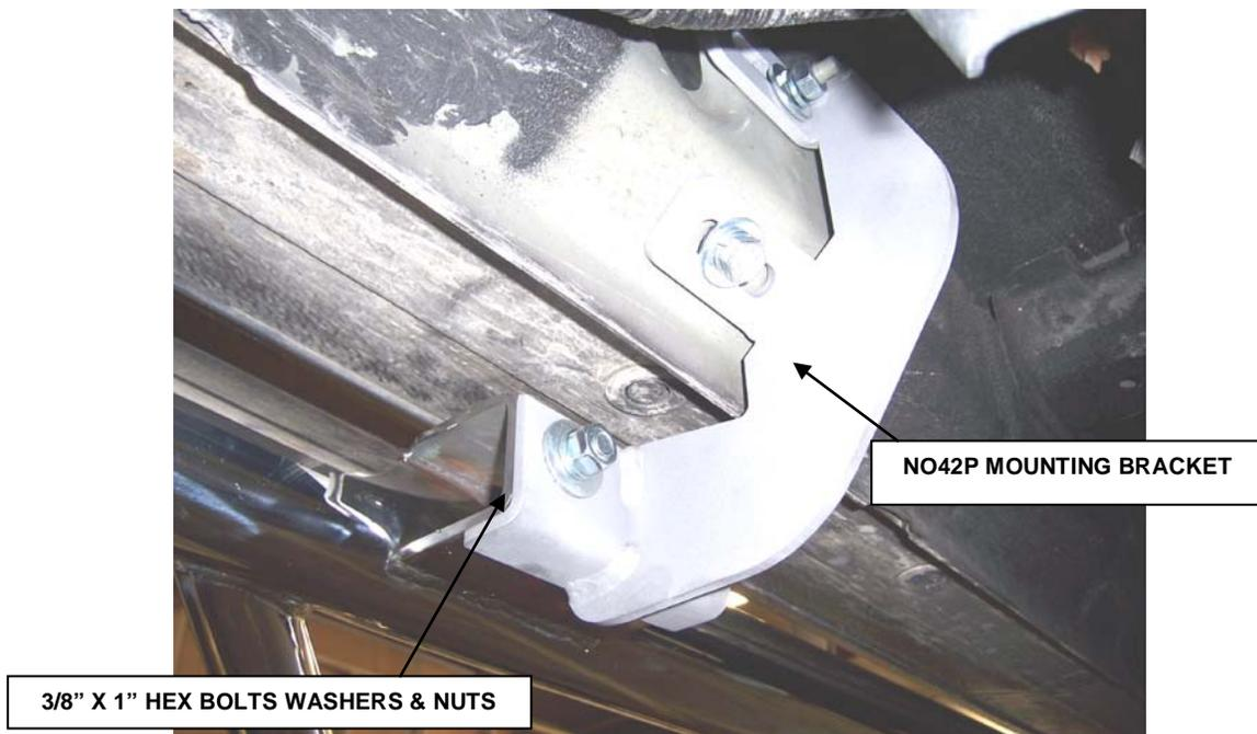
**STEP 4.** Position the passenger sidestep up to the mounting brackets and loosely attach it to the brackets using the 3/8" x 1" hex bolts, washers and nuts as shown.
