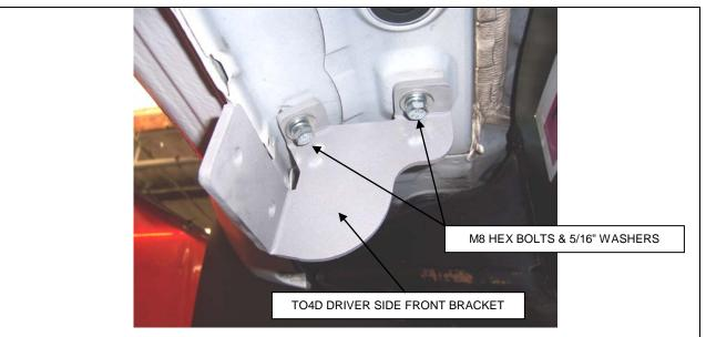
STEP 3. Loosely attach TO4D front bracket to the body panel using the M8 hex bolts, and 5/16" washers.
