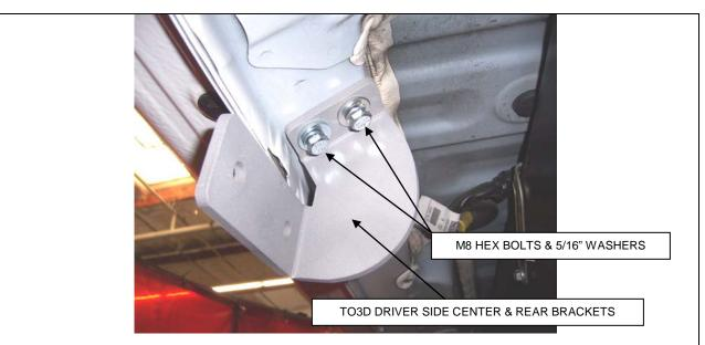
**STEP 5.** Loosely attach the TO3D center and rear brackets, to the body panel using the M8 hex bolts, and 5/16" washers.
