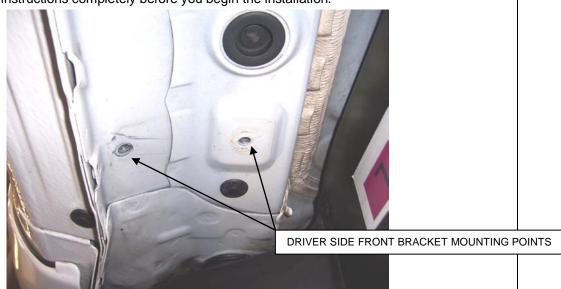
**STEP 2.** This installation uses (3) brackets per side. Begin by installing the driver side front bracket. Locate the (2) threaded holes in the underside body panel.
