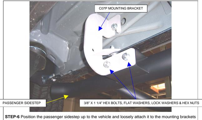
using the 3/8" x 1 1/4" hex bolts, flat washers, lock washers and hex nuts.
