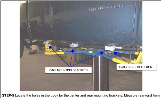
the front fender bolt 37 <sup>3</sup>/<sub>4</sub>" for the center and 67" for the rear bracket. Repeat steps 3 & 4 to install the center and rear brackets.
