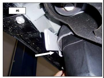
**Step-4** Position the hole in the front of the bracket over the T-Bolt and install (1) 3/8" flat washer, (1) 3/8" lock washer and (1) 3/8" hex nut. Align the hole in the flange of the bracket with the U-Nut and install (1) 5/16" flat washer, (1) 5/16" lock washer and (1) 5/16" x 1" hex bolt. Leave the nut and bolt loose for final adjustment. **Photo #7 & #8**
