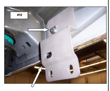
Step-6 Passenger side rear bracket installation.
