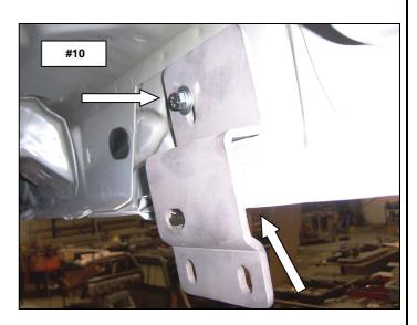
Step-6 Passenger side rear bracket installation.
