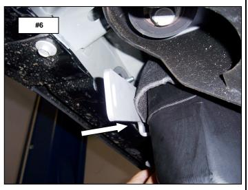
**Step-4** Position the hole in the front of the bracket over the T-Bolt and install (1) 3/8" flat washer, (1) 3/8" lock washer and (1) 3/8" hex nut. Align the hole in the flange of the bracket with the U-Nut and install (1) 5/16" flat washer, (1) 5/16" lock washer and (1) 5/16" x 1" hex bolt. Leave the nut and bolt loose for final adjustment. **Photo #7 & #8**
