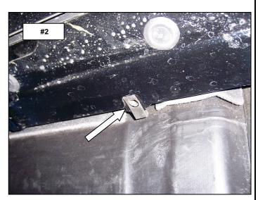
**Step-2** Locate in front of the urea tank the plastic plug in the body rocker panel. Remove the plug, Install the vinyl gasket over the threads of the 3/8" T-Bolt and install T-Bolt in the rocker panel as shown. **Photo #3 & #4**
