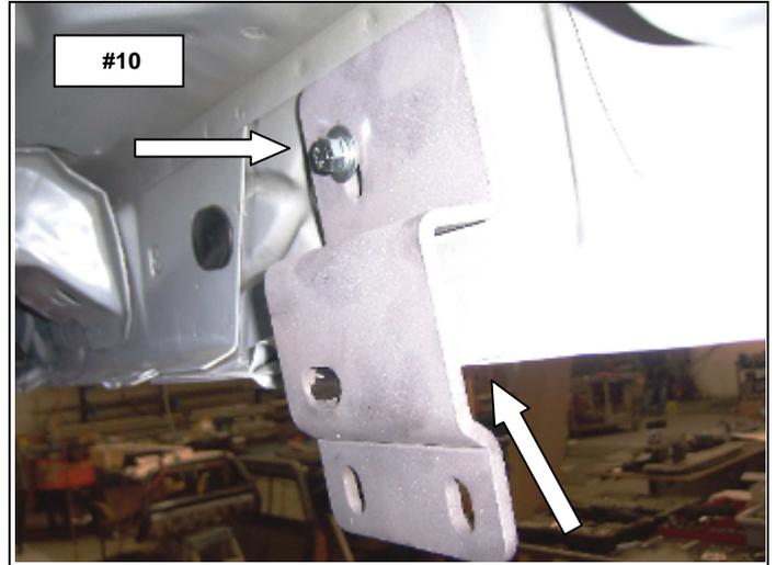
**Step-6** Passenger side rear bracket installation.
