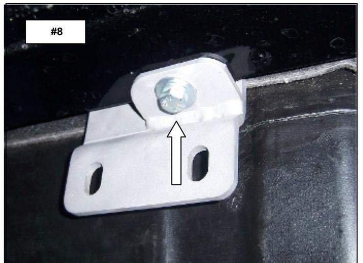
**Step-5** Passenger side Center bracket installation.
