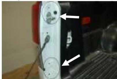
Remove the two phillips screws located directly behind the tail light housing
