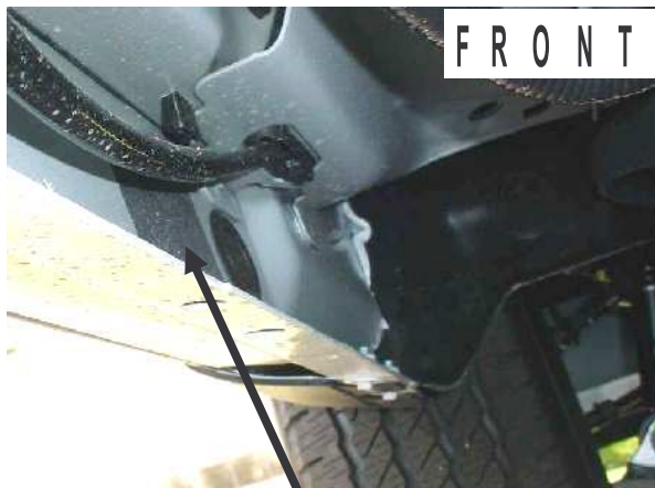
To install front bracket remove this plastic cover . front driver side image.
