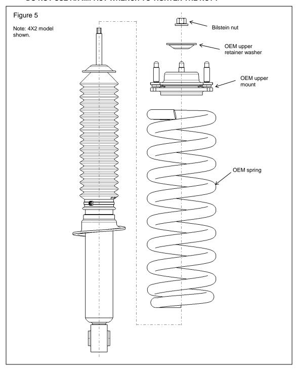
**Q.** Release the spring compressor while ensuring that the ends of the spring remain aligned with the spring seat and upper mount.
