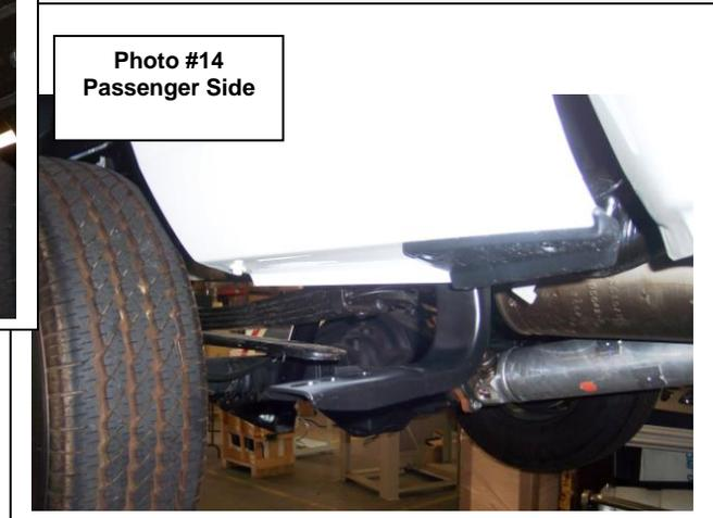
**Step-8** Set the side bar on top of the brackets and align the side bar with the vehicle. Position the clamp brackets inside the opening of the side bar and align the clamp bracket threads with the slot holes in the brackets. Attach the side bar to each of the brackets using the clamp bracket (2) 5/16" x 1" square head bolts, (2) 5/16" lock washers and (2) 5/16" flat washers. **Photo #15**
