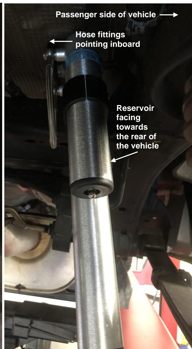
Figure 6. Passenger Side (Rear View)
