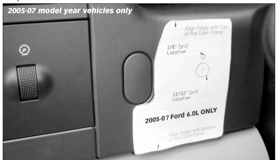
Figure 48 Template taped to front of dash on 2005-07 model year vehicle, ready to be drilled.
