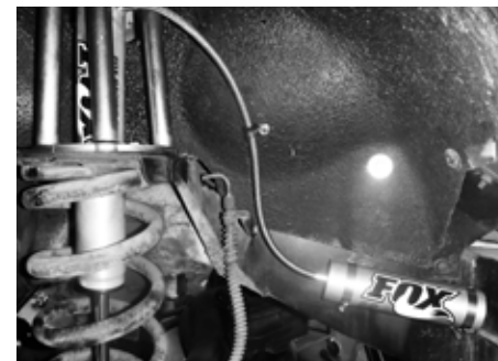
Fig. 4: Driver side remote reservoir mounting
