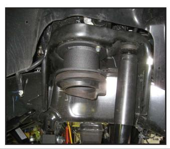
8. Locate the OE coil springs. Working on the driver side, install the coil spring back into the vehicle. Carefully raise up on the hydraulic floor jack until the coil spring seats properly into the newly installed isolator and coil spring spacer. Repeat procedure on the passenger side.
