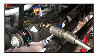
4. Remove the bolt from the track bar where it attaches to the driver side frame bracket. Save the hardware and remove the entire front track bar.
