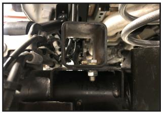
(2) 1/2" unitorque nuts. Apply a lithium based grease to the 75 ft lbs. bushings and install them into the eyelets of the new sway
