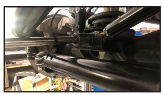
24. With the front track bar installed, tilt it slightly towards the front bumper and tighten the 2 jam nuts on each heim joint
