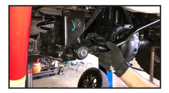
35. Remove both rear shock absorbers, and save the mounting hardware.
