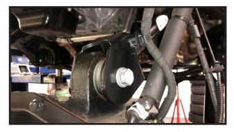
18. Install the new lower control arm using the OE hardware.
