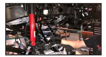
13. Working on the driver side, remove the heat shield from the upper control arm frame mount pocket
