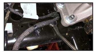
28. Install new front shock absorbers using the OE hardware. Special note: if your new front shocks do not have the proper upper bushings and sleeves already installed in them, make sure to use the new S10325 shock spacer sleeves from hardware bag 44105NB1
