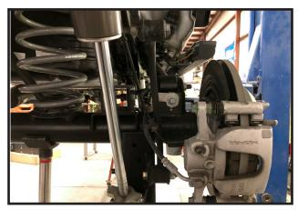
59. Install new rear shock absorbers using the OE hardware. Special note: if your new rear shocks do not have the 57. Locate (2) new rear sway bar end links, part # F2355-proper upper bushings and sleeves already installed in 02. Also locate (8) MO2220 bushings, (4) S10026 crush them, make sure to use the new S10325 shock spacer sleeves, (2) 1/2" x 2 1/2" bolts, (4) 7/16" flat washers and sleeves from hardware bag 44105NB1. Torque bolts to
