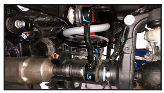
9. Working on the passenger side, locate and remove the brake hose bracket that is attached to the lower coil spring perch. Save hardware
