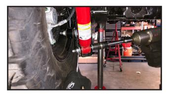
36. Located on the outside of the frame rails, are the brake hose brackets, you will need to remove the bolts that are attaching them to the frame. Save the bolts
