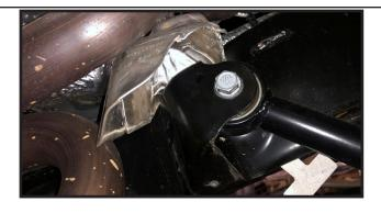
Remove the upper control arm from the vehicle and save the mounting hardware
