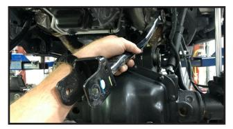
15. Working on the driver side, remove the lower control from the vehicle. Save the hardware
