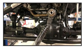
5. Remove both of the front shock absorbers from the vehicle. Save all of the hardware. Special note: these photos only show removing the lower shock hardware, but you will need to remove the shock completely.
