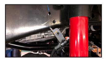
7. Carefully pry open the metal brake hose brackets that are attached to the lower control arms so that the rubber brake hose can be removed. This step needs to be performed on driver and passenger side.
