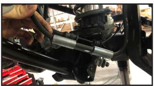
10. To obtain slack in the wire harnesses that control the front axle, you will need to pop out some plastic plugs. these are located on both upper control arms where they mount to the axle, and also up on the inner frame rail if you follow the wires up. Take special care to not damage any wires or plastic plugs as they will get re-installed later on.
