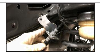
37. Located on the passenger side of the rear axle is the breather hose, and it is clipped to the emergency brake cable and electric rear locker wire harness. You will need to unclip enough of these clips to gain slack to lower the rear axle down. See photos below
