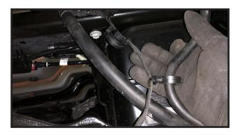
38. With all the gained slack in the brake hoses, and wire harness, carefully lower the rear axle down enough to remove both rear coil springs. Save the upper rubber coil spring isolator.
