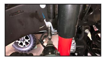
31. Working on the REAR of the vehicle, remove the OE sway bar end links and install them on the FRONT of the vehicle. Use the OE hardware and torque to 65 ft lbs.
