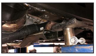
12. With all the slack now obtained in the wire's and brake hoses, carefully lower down the front axle and remove the front coil springs. **Take special care to not over extend any wires or brake hoses.**
