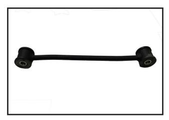
55. Locate (2) new rear bump stop brackets, part # 44100-¶58. Using the OE hardware on the top eyelet and the new 09. Also locate (4) 3/8" x 1 1/4" bolts, (4) 5/16" flat washers, 1/2" hardware on the bottom eyelet, Install the new end links making sure that they match the following photos. Torque bolts to 75 ft lbs.
