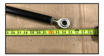
23. Install the S10336 mis-alignment sleeves into each heim joint and install the new track bar in the vehicle using the OE mounting hardware. Torque bolts to 125 ft lbs. Special note, if the track bar does not line up to the mounting holes right away, you may need to pry the axle side to side to get it aligned.
