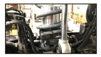
21. Install the 3/8" flange nut on the 3/8" x 3/ 1/2" bolt and torque to **30 ft lbs.**
