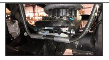
27. Re-install the wire harness plugs/clips to the upper con- 30. Re-install the brake hose brackets to the driver and pastrol arms and the frame rails.
