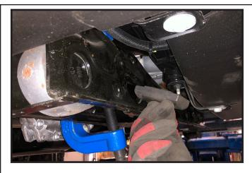
10. tap the torsion bar forward until the torsion bar key can be removed.
