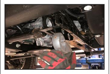
11. Locate the new torsion bar key and install it making sure to line up your reference marks on the torsion bar and lower control arm.
