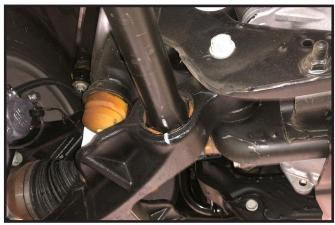
8. Working on the driver side, remove the torsion bar adjustment bolt and set aside.
