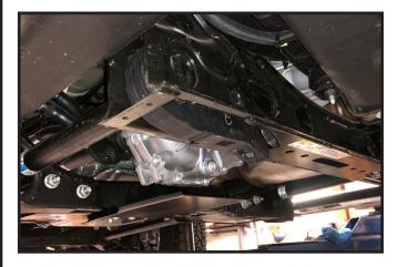
12. Using a proper torsion bar removal tool. Special note: Tuff Country EZ-Ride Suspension requires that a proper torsion bar unloading tool be used when performing this installation. Carefully load the torsion bar up enough to re-install the adjusting block and bolt.
