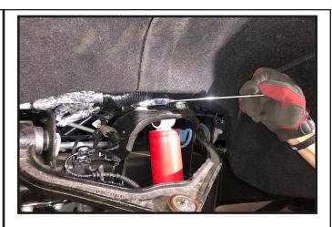
4. Carefully compress the shock absorber enough to slide the new spacer sleeves over each shock bolt, and then let the shock retract back into its original location.
