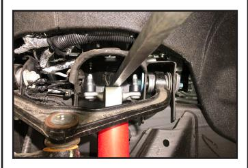
5. Install the new supplied shock nuts onto the OE bolts and torque to **65 ft lbs**.
