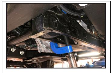
13. Adjust the bolt up until it is to is OE position (typically about 1/2 way in). Final height adjustments will be made at the end of the installation with the vehicle sitting on the ground.
