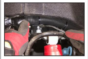
3. Remove the OE nuts from the shock bolts and discard.
