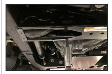
9. Using a proper torsion bar removal tool. Special note: Tuff Country EZ-Ride Suspension requires that a proper torsion bar unloading tool be used when performing this installation. Carefully remove the stock torsion bar bolt and block, and set aside. Remove the torsion bar unloading tool from the crossmember.
