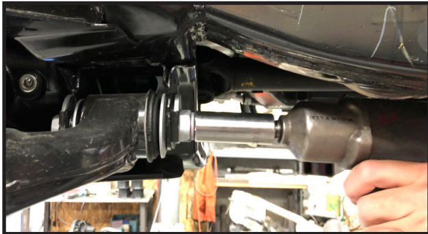
13. Remove lower strut mount hardware on driver and passenger side. Save hardware.
