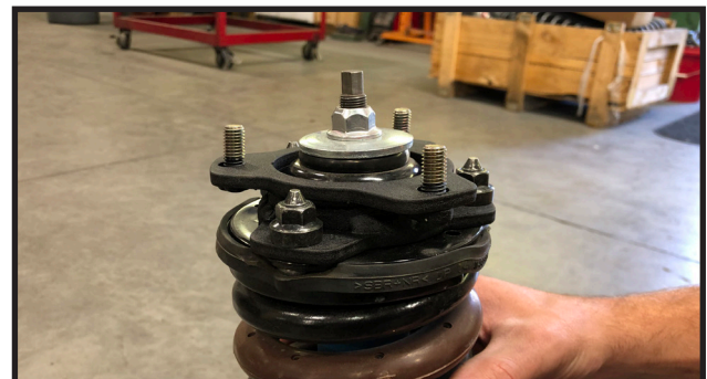
17. Locate part # 52915-01 and the three OE upper strut nuts. And install on to the strut. Tighten to 36 ft-lb. Special note. If OE strut studs are higher than the new spacer. Grind off the tip of the studs.
