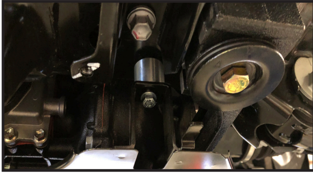
12. Working on driver side. Loosen the front and rear cam bolts on the lower control arm. Repeat on passenger side.
