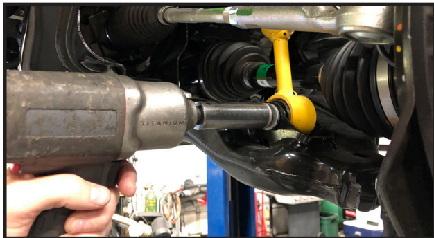
14. Remove the three nuts on the top strut mount. Save hardware.
