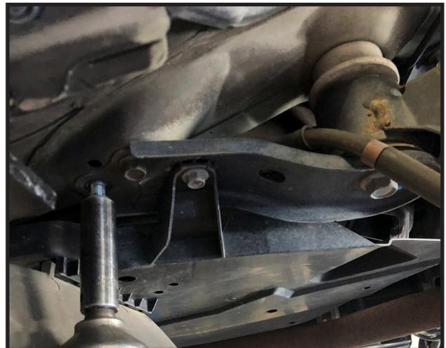
16. Locate the (4) main subframe mounting bolts and remove them. These are located at each corner of the rear subframe.
