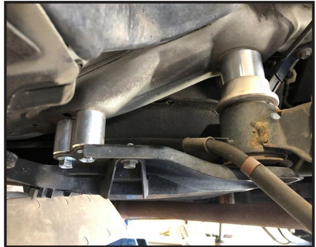
23. Torque the (4) 14mm subframe bolts to 100 ft lbs.
