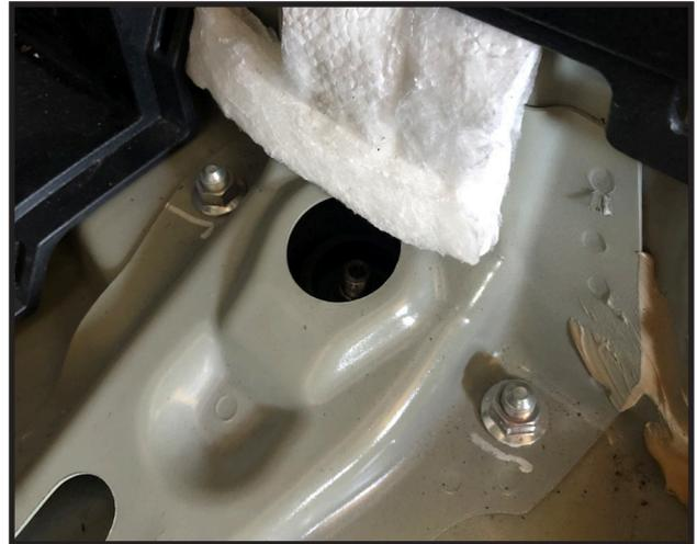
15. Working under the rear of the vehicle, Locate the trailing brackets on both the driver side and passenger side. Remove the 2 bolts that attach them to the body of the vehicle.
