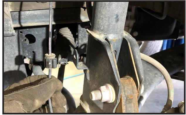
4. Remove the 2 bolts that attach the strut to the steering knuckle and carefully lean the steering knuckle out of the way.
