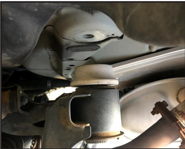
17. Remove the lower strut mounting bolts and completely remove the struts from the vehicle.
