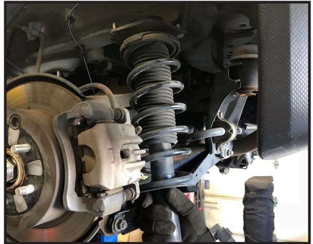
18. Take the struts to the work bench or vice and carefully hammer out the OE studs from the top of the strut.
