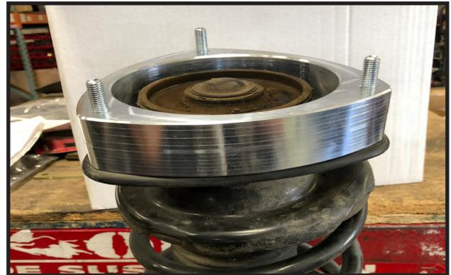
8. Re-install the strut into the vehicle using your marks to make sure it is in the same orientation that it was removed from. Secure using the OE nuts. Torque to 28 ft lbs.
