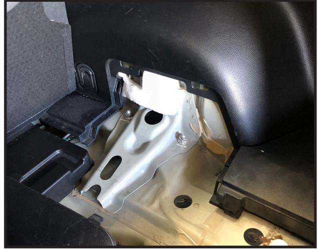
14. You should see the 2 upper strut mount nuts. Remove them from both the driver and passenger side rear struts.
