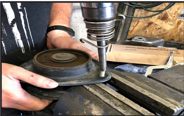
7. Locate the new 51700-01 strut spacer and install it on the top of the strut plate making sure to line the 3 holes up. Secure the new spacer using the 3 new 8mm x 60mm bolts. Torque bolts to 28 ft lbs.
