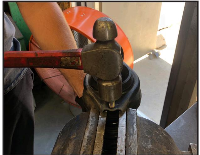
19. Locate the new 51700-02 rear strut spacers and also locate (4) 10mm x 60mm bolts. Install the new spacers on the top of the struts using the new metric bolts. Torque bolts to 35 ft lbs.
