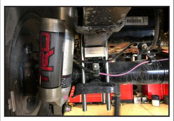
32. Carefully remove the jack from underneath the leaf spring and repeat on the opposite side of the vehicle.
