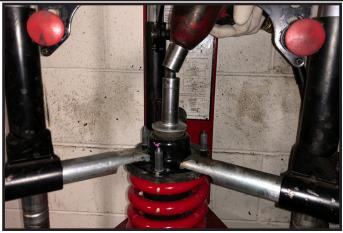
15. Remove the strut assembly from the strut compressor and take it back over to the vehicle.
