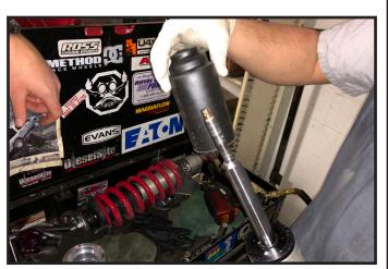
11. Locate a new strut spacer part # 51020-01 and install it over the body of the shock. **Make sure to install the new spacer so that the "coil shelf" is facing upwards.**
