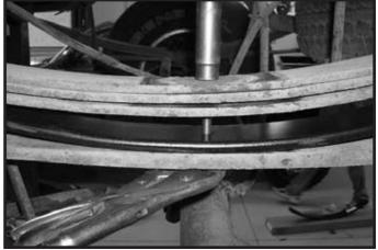
cut off the excess thread from the new centering bolt.
