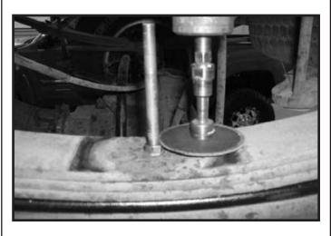
42. Secure the axle to the spring pack using the new u-bolts, u-bolt hardware and stock u-bolts plates. Special note: If the rear u-bolts are 1/2", torque to 52 - 70 ft lbs. 9/16" torque to 75 - 100 ft lbs. 5/8" torque to 107 - 143 ft lbs. 3/4" torque to 190 - 253 ft lbs.
