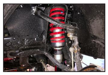
17. Raise the lower control arm back up until you can install the OE lower mounting bolt and hardware. Leave this loose for now.
