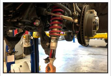
Tuff Country EZ-Ride Suspension recommends a wall mounted strut compressor be used when performing the steps that talk about installing the spacer into the strut. If you do not have a wall mounted strut compressor, please have these steps performed by your local Toyota Dealership
