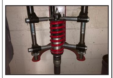
Carefully compress the strut until the upper hardware can be removed. Remove the nut and hardware and save for re-assembly.
