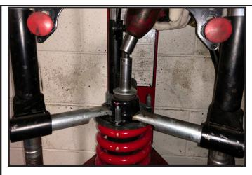
10. Remove the shock absorber from the strut assembly out of the bottom of the coil spring. Remove the metal washer and plastic dust boot. Save for re-installation
