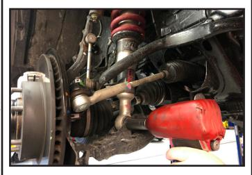
5. Locate and remove the 2 bolts that attach the lower control arm ball joint piece to the steering knuckle.
