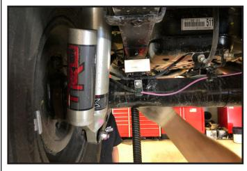
31. Locate the new rear u-bolts along with the new nuts and washers. Install the u-bolts and torque them to 150 ft lbs.
