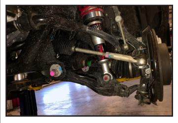
18. Raise the lower control arm up even more until you can re-install the 2 lower ball joint bracket bolts to the steering knuckle. Torque to 160 ft lbs.
