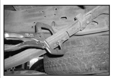
39. Carefully remove the centering bolt and discard. **Special** note: Once the centering bolt has been removed, the overload spring will fall out. Save the overload.
