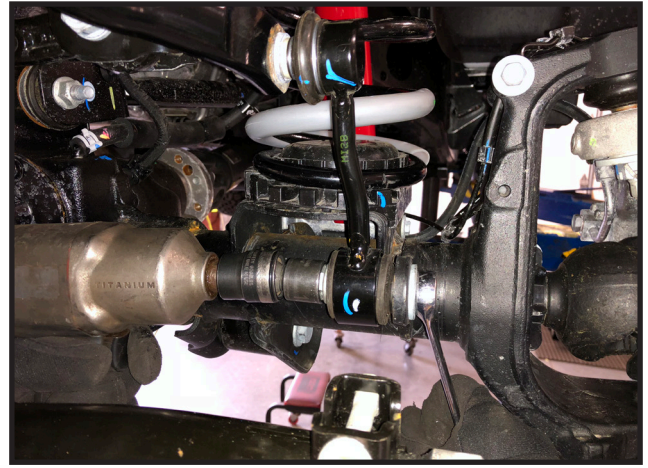
6. Working on the driver side inner frame rail, just behind the steering gear box, locate and remove the plastic plugs holding the wire harness to the frame. This is done to gain slack in the wires during the install process.
