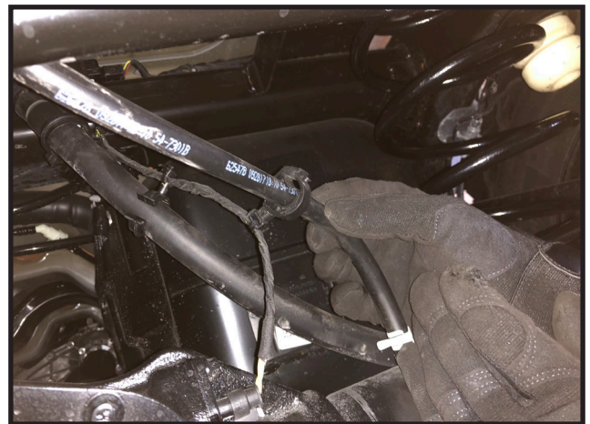
23. Working on the passenger side, you can see the wire harness is attached to the axle breather hose in multiple locations. You will need to remove these attachment points to gain slack in the wire harness for this install process.
