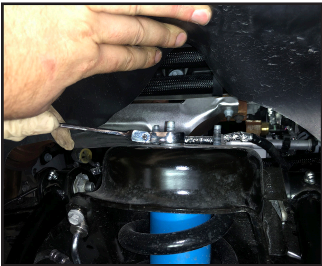
12. Remove 2 of the 3 upper strut mount nuts and loosen the 3rd one.
