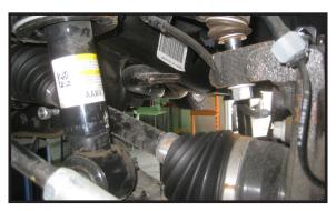
7. You should now have enough space between the lower 12. Re-install tires and wheels. strut mount to install the new 12002-01 spacer. Install or both sides of the vehicle.
