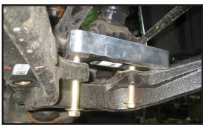
8. Locate (4) 10mm x 1.5 x 80mm bolts if your lower control arm is made of steel, and (4) 10mm x 1.5 x 90mm bolts if your lower control arms are made of aluminum. Also locate (8) 10mm washers and (4) 10mm unitorque nuts. Install the new hardware to secure the lower strut mount with the newly installed 12002-01 spacers. Torque to 35 ft lbs.
