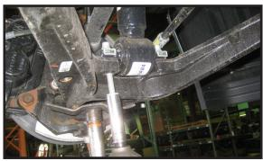
4. On both sides of the vehicle, remove the nut clips from the lower strut mounts and discard.
