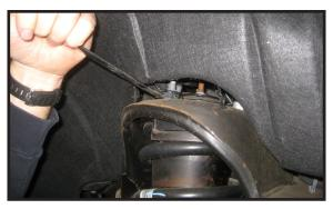
6. Working on the driver side, loosen, but DO NOT remove the upper control arm nut. Using a hammer, carefully hit the steering knuckle to break the ball joint taper free. Repeat on passenger side.
