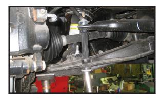
Working on the driver side, remove the bolts attaching the lower strut to the lower control arm, discard bolts and repeat on passenger side.
