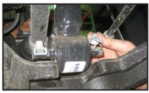
Working on the driver side upper strut mount, loosen the 3 nuts. It is not necessary to completely remove them. Repeat on passenger side
