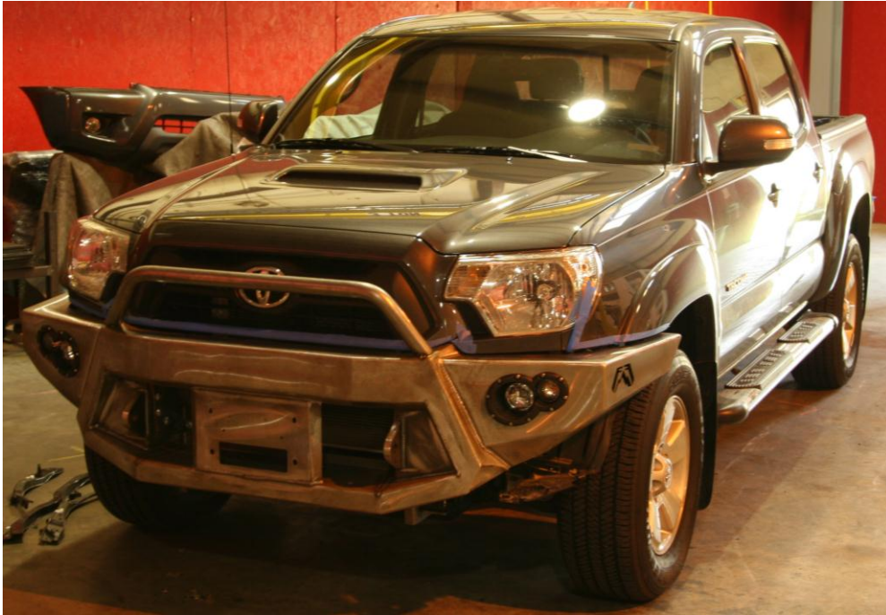
Figure 21 – Completed bumper installation (shown with PreRunner tube option)
