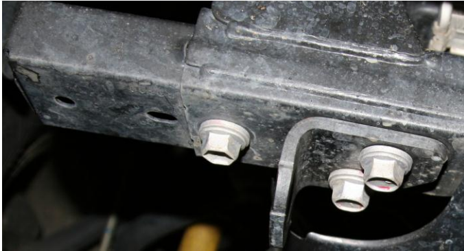
Figure 11 & 12 – Bumper beam extension and tow eye removal
