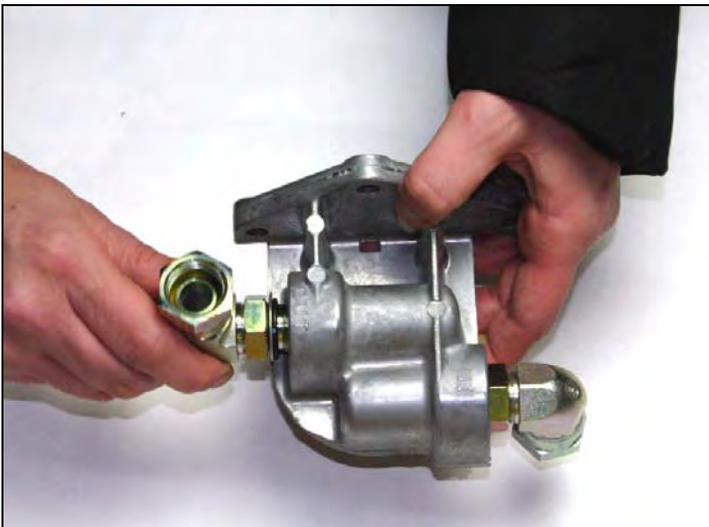
Install the two **90° ORB fittings** (1604046) into the filter head (do not use pipe sealant). When installed, the fittings need to point toward the front of the vehicle. For ease of installation, we recommend assembling the fittings on the filter head on a work bench before installing it onto the vehicle.
