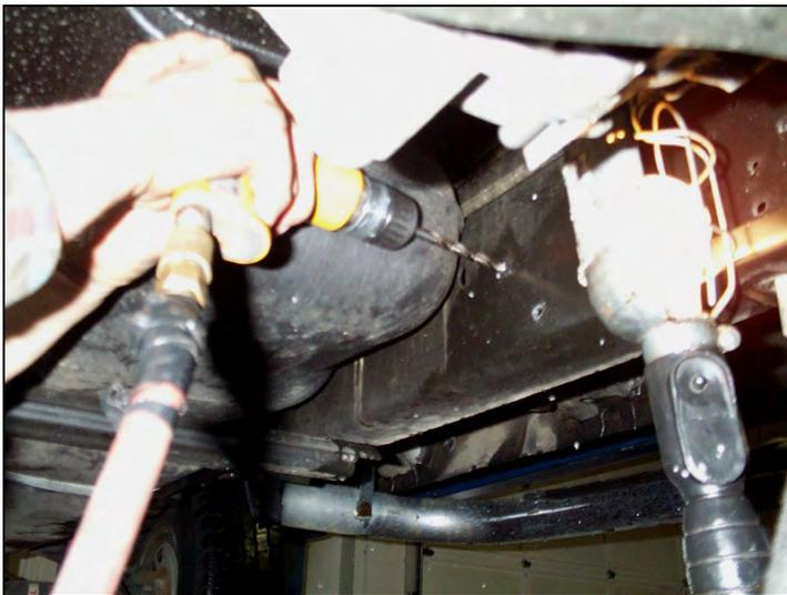
Using a small sized drill bit (1/8"), drill a pilot hole for each bolt hole then enlarge the hole with a 3/8" drill bit.
