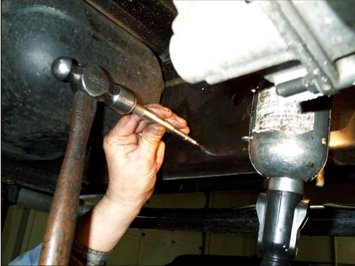
To allow for easier drilling, center-punch the two marked spots for the three mounting bolts.
