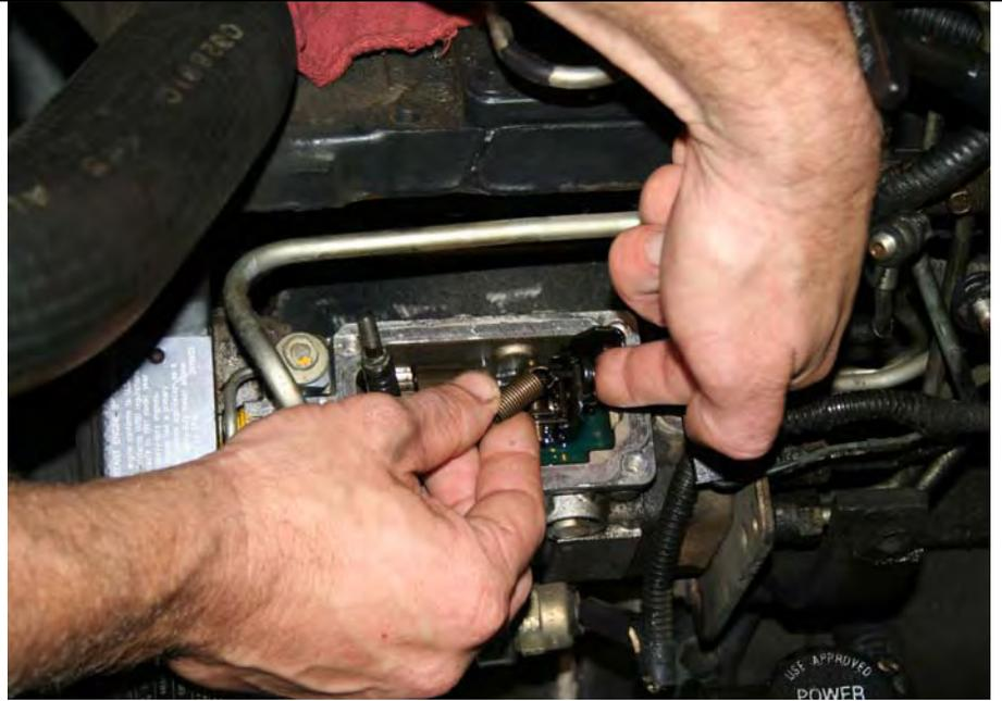
12. Replace oring on throttle shaft, with the oring supplied (#1505020).
