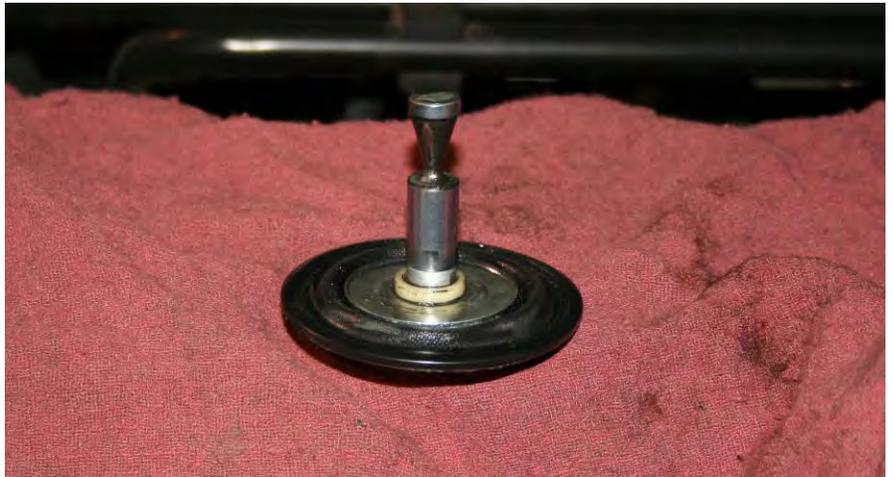
7. Remove the factory fuel pin from the diaphragm by using two 10mm wrenches. One on the jam nut the other on the rectangular slots on the fuel pin.
