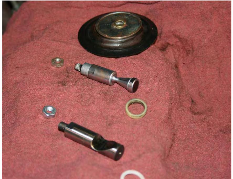
9. Before inserting new pin assembly, stroke the throttle linkage back and forth slightly. You can use some lubrication at the same time to assist you.
