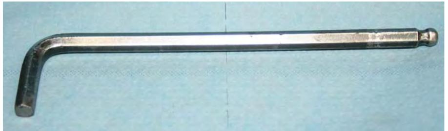
9. Using the rounded end of the allen key remove the 4 bolts holding the cover on. You will need to use a wrench on the end of the allen key as the bolts are quite tight.
