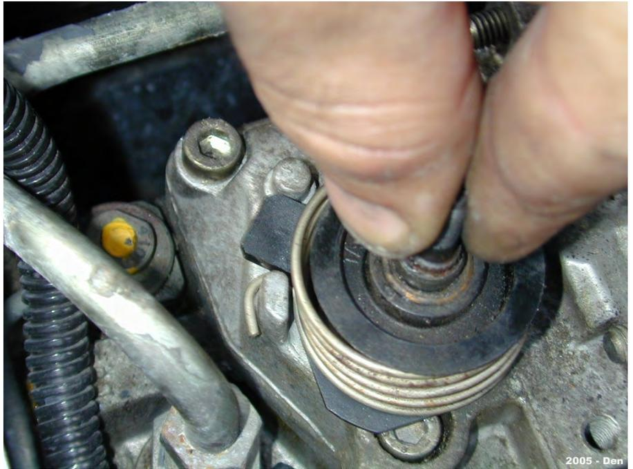
16. Now tighten the main fuel screw back in to the previous position.
