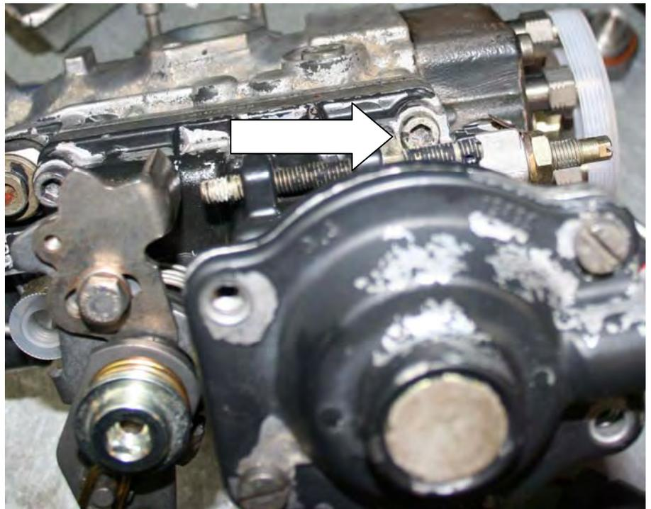
10. With the 4 bolts removed pull up on the cover while pushing down on the throttle shaft.
