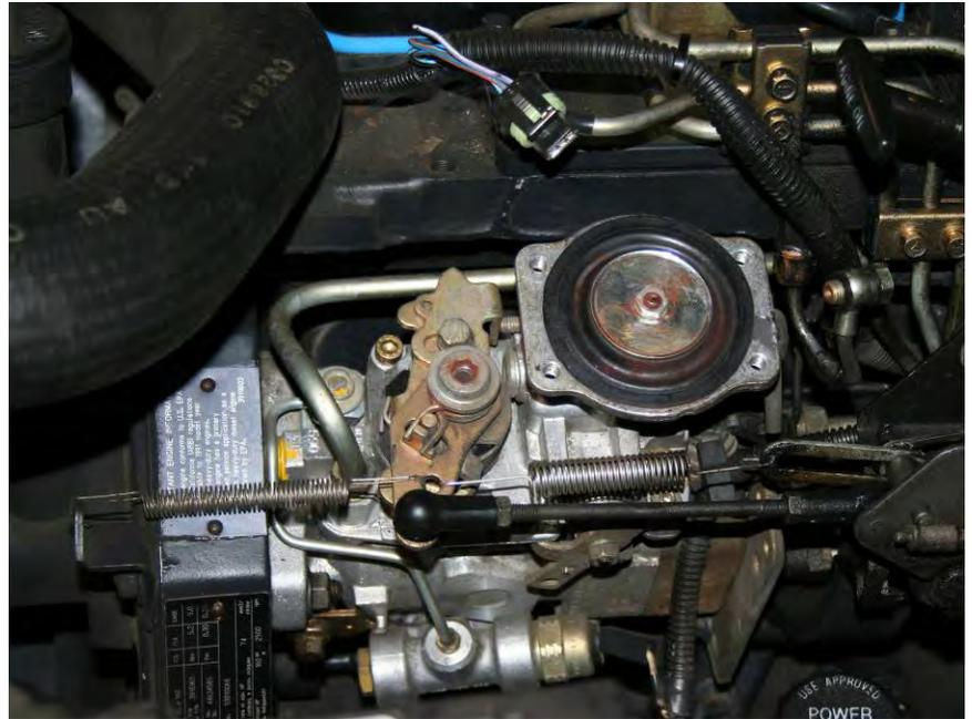
6. Remove the factory white nylon bushing. It may be stuck to the bottom of the diaphragm, or at its base in the fuel pump.
