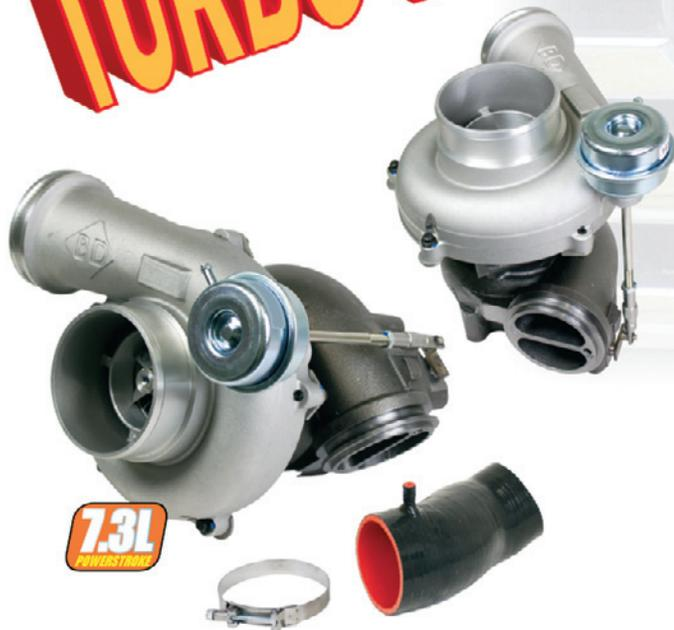
BD uses their own version of thrust collar and back plate as well their own designed sintered brass 360-degree 6-pad thrust bearing that reduces heat build-up and increases durability. Using a proven 66/88 mm compressor wheel that is HIP'd (Hot Isostatic Pressed) improves centrifugal strength at high rotating speeds and boost pressures. BD's exclusive Heavy Duty Waste Gate controls maximum boost pressure.
