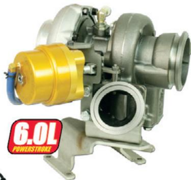
BD's Turbo Thruster upgrade kit for the 2003-2007 6.0L Power Stroke delivers the kind of power late-model Ford truck owners have been looking for! Featuring the Borg Warner S300 turbocharger with extended tip technology, double-port adjustable waste gate and shrouded housing, this turbo delivers quick response with strong mid and top-end power.
