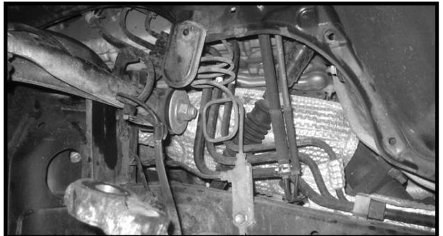
14. Working on the driver side, remove and save the hardware attaching the upper control arm to the OE location. The upper control arm may be discarded. Repeat procedure on the passenger side.
