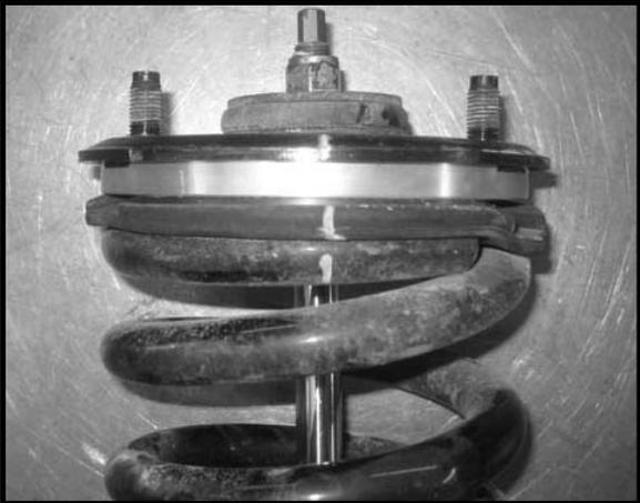
19. Locate the new upper strut spacer. Install the new upper strut spacer to the modified strut and secure using the OE hardware. Make sure to use loctite and torque to **45 ft. lbs.** Place the driver side strut aside for later installation into the vehicle.
