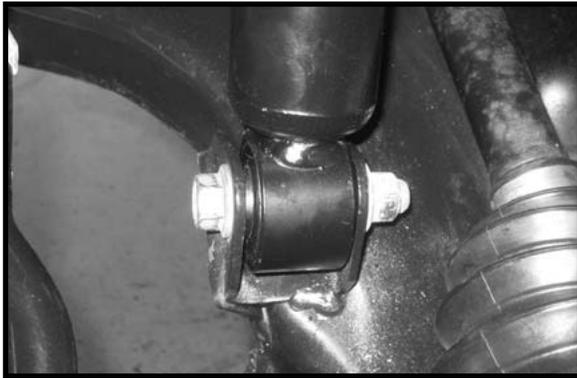
23. Working on the driver side, move back to the 3/8" hardware and add some loctite and torque the (3) nuts to **28 ft lbs**. Repeat procedure on the passenger side.
