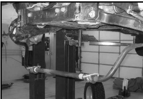
4. Locate the new sway bar relocation brackets. Also, locate (4) 7/16" x 1 1/4" bolt and (4) 12 mm x 30 mm socket head bolts from hardware bag 54060NB. Install the new 7/16" x 1 1/4" bolts to the new sway bar brackets into the cut out slot.
