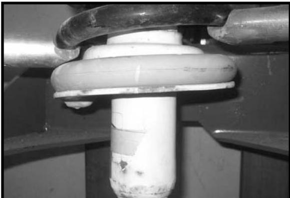
14. Place a clamp on the bottom coil portion of the coil spring and strut plate. This will help keep the coil spring in the proper location.
