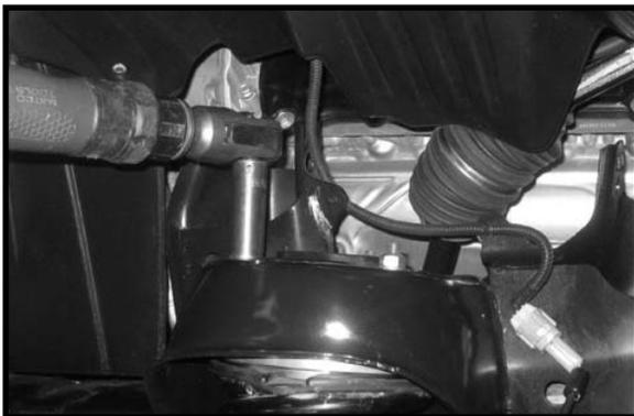
24. Locate the new upper control arms. Locate (8) poly bushings and (4) S10243 sleeves from hardware bag 54060PL. Install the new bushings and sleeves into the new upper control arms. **Special note: Make sure to use a fair amount of lithium or moly base grease before installing the new bushings and sleeves into the control arms. This will increase the life of the bushing as well as help prevent squeaking.**
