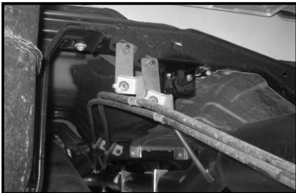
47. Carefully lower down on both hydraulic floor jacks at the same time until the springs separate from the rear axle. Lower down approximately 4". **Special note: Make sure not to over extend any brake lines or hoses when lowering axle.**
