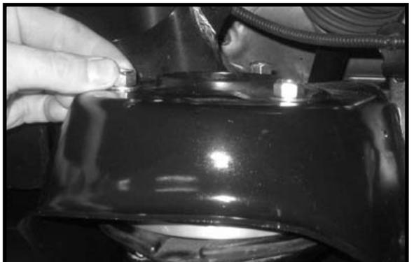
22. Working on the driver side, secure the bottom portion of the strut to the lower control arm using the OE hardware. Make sure to use loctite and torque to **150 ft lbs**. Repeat procedure on the passenger side.
