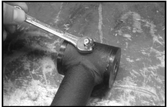
26. Working on the driver side, install the new upper control arm into the upper pockets using the OE hardware. **Do not tighten at this point.** Repeat procedure on the passenger side.
