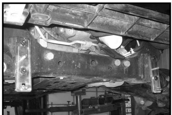
5. Locate (4) 3/8" USS flat washers and (4) 7/16" unitorque nuts from hardware bag 54060NB. Working on the driver side, attach the sway bar to the newly installed sway bar bracket and secure using the new 7/16" hardware. Make sure to use loctite and torque to **40 ft lbs.** Repeat procedure on the passenger side.
