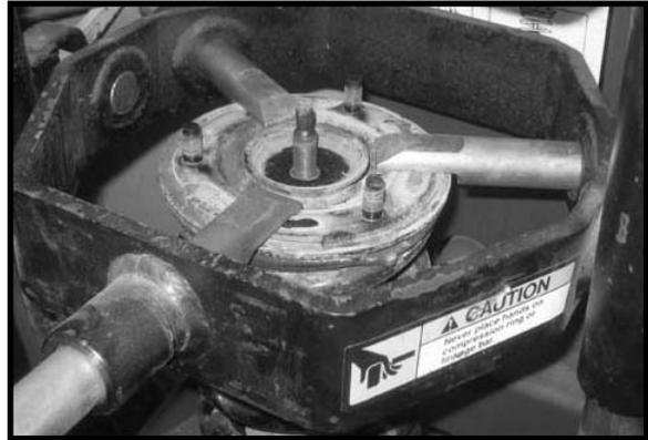
16. Carefully loosen the wall mounted strut compressor until the bearing plate can be removed from the coil over.
