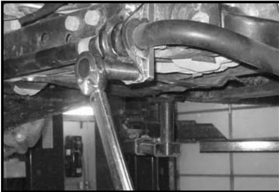
6. Place a pair of hydraulic floor jacks under the driver and passenger side lower control arm. Carefully raise up on both hydraulic floor jacks until they come into contact with the lower control arms.
