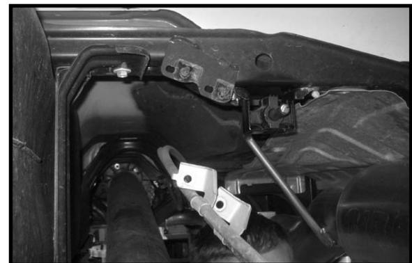
45. Locate (2) emergency brake line relocation brackets from hardware bag 54060NB1. Install the new brackets to the OE location using the OE hardware. Make sure to use loctite and torque to **12 ft lbs.**
