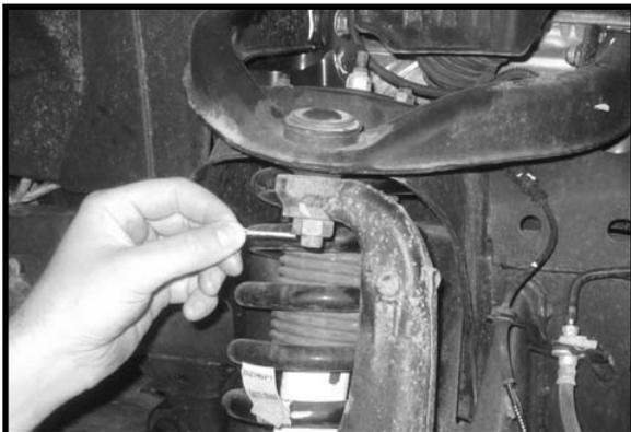
8. Working on the driver side, loosen but do not remove the castle nut holding the upper control arm to the knuckle. With a hammer, carefully hit the knuckle to break the taper. Once the taper has been broken, remove the castle nut and discard. Separate the upper control arm from the knuckle. Repeat procedure on the passenger side.
