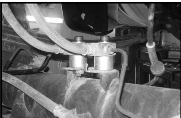
43. Working on the driver side, remove the rear u-bolts. The rear u-bolts and hardware may be discarded. Set the stock lower u-bolt plate aside for later re-installation. Repeat procedure on passenger side.
