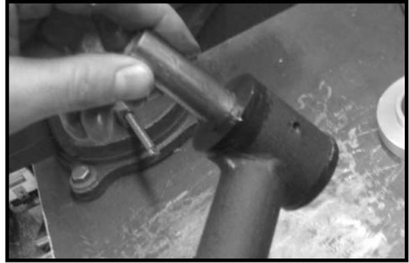
25. Locate the new sert fittings from hardware bag 54060PL. Install the new sert fittings into the new upper control arms. **Special note: Make sure not to over tighten and also make sure that the sert fitting is facing towards the outside of the vehicle. This will make for easier access when using a grease gun.**
