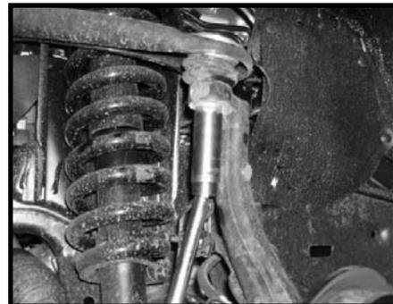
7. Working on the driver side, remove the stock cotter pin from the stock outer tie rod ball joint. Save the stock cotter pin. Repeat procedure on the passenger side.
