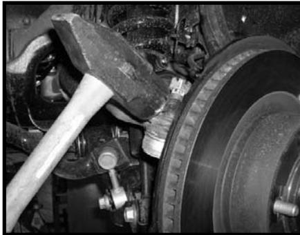
9. Move back to the stock upper control arm ball joint nut and remove completely. Also, move back the stock outer tie rod ball joint nut and remove completely. Remove the stock upper control arm and the stock outer tie rod from the stock knuckle. Let the stock knuckle hang. **Special note: Make sure not to over extend the brake lines, ABS lines and the stock CV axle, if need be, tie the stock knuckle up so these problems do not occur.** Repeat procedure on the passenger side.
