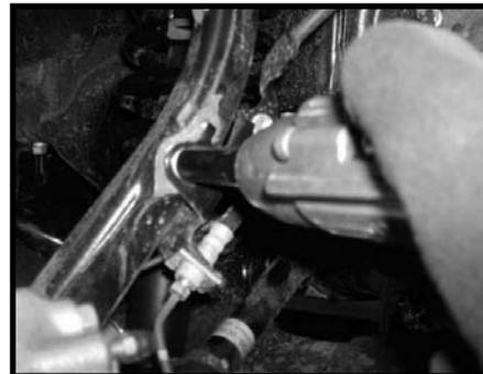
28. Locate the stock ABS mounting hardware. Working on the driver side, secure the stock ABS bracket to the stock upper control arm and secure using the stock hardware. Make sure to add some thread locker or loctite and torque to **12 lbs.**
