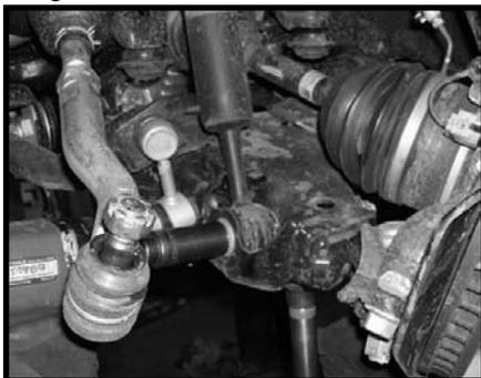
12. Working on the driver side, remove the stock sway bar end link hardware that connects the stock sway bar end link to the stock lower control arm. Save the stock hardware. Repeat procedure on the passenger side. Let the stock
