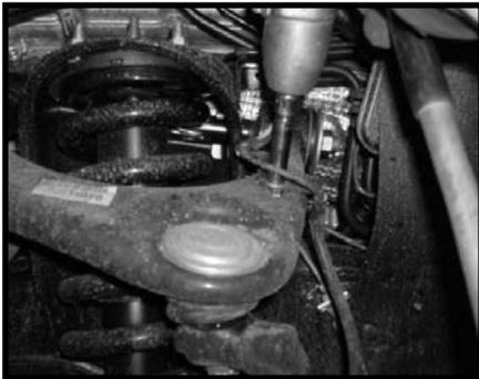
3. Working on the driver side, remove the stock hardware that connects the stock brake line bracket to the stock knuckle. Save the stock hardware. Repeat procedure on the passenger side.
