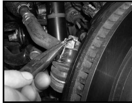
27. Locate the stock brake line mounting hardware. Working on the driver side, secure the stock brake line bracket to the stock knuckle and secure using the stock hardware. Make sure to add some thread locker or loctite and torque to **12 lbs.**
