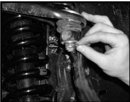
25. Locate the stock outer tie rod castle nut. Working on the driver side, install the stock outer tie rod to the stock knuckle and secure using the stock castle nut. Make sure add some thread locker or loctite and torque to **67 lbs.**
