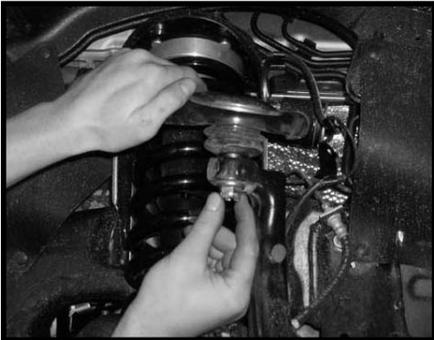
24. Locate the stock upper control arm cotter. Working on the driver side, install the stock cotter back into the stock upper control arm ball joint. **Special note: If the stock cotter pin can not be installed because the hole in the stock castle nut does not line up with the stock ball joint, DO NOT loosen the stock castle nut so that the cotter pin can fit, tighten the stock castle nut some more so that the stock cotter pin can be installed.**
