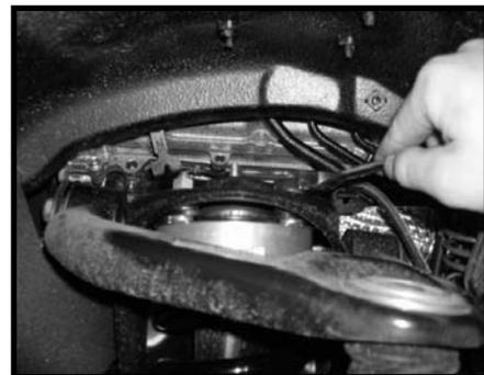
19. Locate the stock sway bar end link mounting hardware. Working on the driver side, secure the stock sway bar end link to the stock lower control arm using the stock hardware. Add some thread locker or loctite and torque to **60 ft lbs.**
