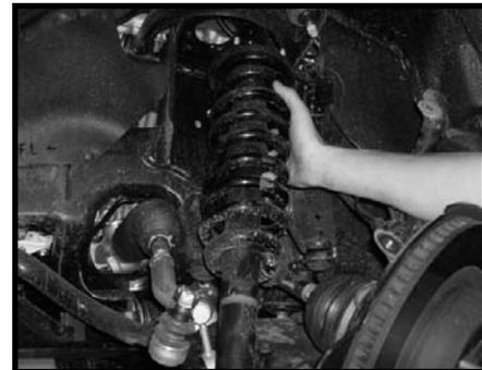
14. Working on the driver side strut, measure the exposed threads sticking out of the middle bolt on the stock strut. Repeat procedure on the passenger side strut.
