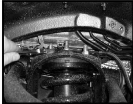
5. Working on the driver side, remove the stock cotter pin from the stock upper control arm ball joint. Save the stock cotter pin. Repeat procedure on the passenger side.
