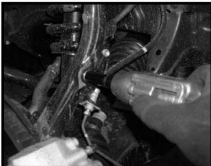
4. Working on the driver side, remove the (4) stock upper outer nuts that connect the stock strut into the stock location. Save the stock nuts. Repeat procedure on the passenger side. **Special note: Only remove the (4) stock upper outer nuts, DO NOT remove the stock nut in the middle of the stock strut.**
