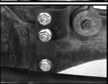
28. Position a pair of hydraulic floor jacks under the rear differential. Place one jack stand on the driver side and one on the passenger side. Raise up on both hydraulic floor jacks at the same time until they make contact with the rear differential. Working on the driver side, remove the rear u-bolts. The rear u-bolts and the u-bolt nuts may be discarded, save the u-bolt washers. Place the u-bolt plate and the bump stop aside for later re-installation. Repeat procedure on the passenger side.
