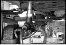
25. Remove the rear brake proportioning valve bracket from the rear axle. The hardware may be discarded.
