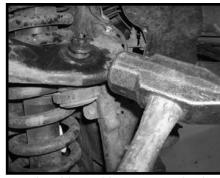
5. Working on the driver side, remove the lower bolt that connects the strut to the lower mounting location and save the hardware for later re-installation. Special note: During removal of the bolt, take special care not to damage the CV boot. Also, make a mental note on which way the bolt is removed, it needs to be re-installed the same way that it was removed. Remove the strut assembly from the vehicle and set aside. Repeat procedure on the passenger side.
