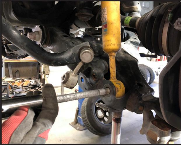
12. Remove the 4 upper strut mounting nuts. **Special note: make sure the lower control arm is properly supported so the suspension doesn't drop out when these nuts are removed.**
