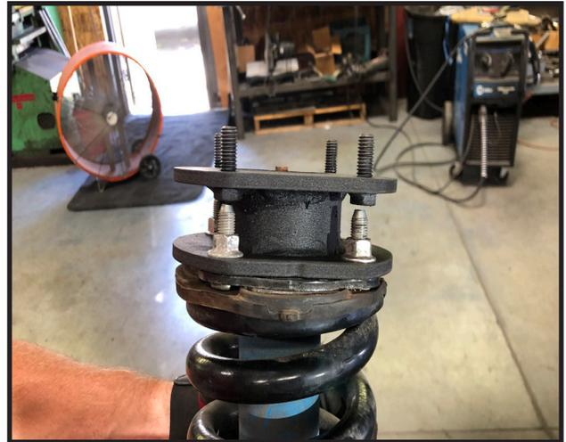
16. Locate the new 3/8" flange nuts, Reinstall the struts back into the vehicle and loosely start the new 3/8" flange nuts. Do not tighten at this time.
