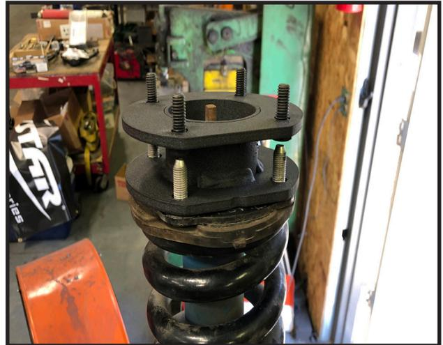
15. Secure the new spacers using the OE nuts
