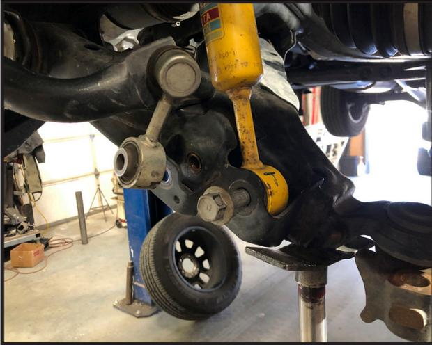
18. Carefully raise the lower control arm up so that the lower ball joint bolts can be re-installed into the steering knuckle. **Torque to 160 ft lbs. Special note: While performing this step, it requires the front suspension to be compressed greatly, so its recommended that a stabilizer jack be placed under the rear bumper or trailer hitch of the vehicle to prevent it from pivoting.**
