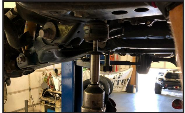
4. Carefully lower the front differential down approximately 3/4" to install the new spacer sleeves.
