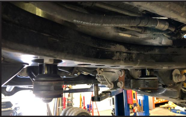
7. Loosen but DO NOT remove the 4 lower control arm cam adjustment bolts.
