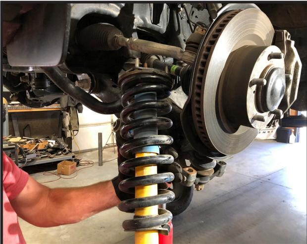
14. Locate the new upper strut spacers part # 52075-01 and install them on top of the OE struts. **Special Note: these spacers only fit on one way and should be installed so the notch is facing outwards of the vehicle.**
