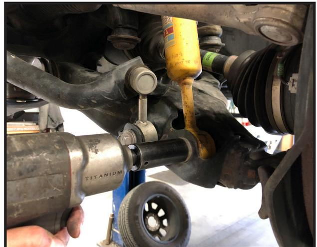
10. Remove the 2 bolts that attach the lower ball joint to the bottom of the steering knuckle.
