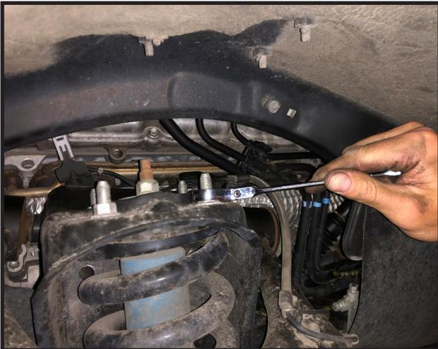
13. Carefully lower down the lower control arm so that the strut assembly can be removed from the vehicle.
