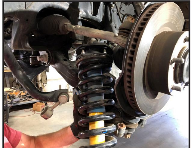
17. Raise up the lower control arm so that the lower strut bolt can be reinstalled, Do not tighten at this time.
