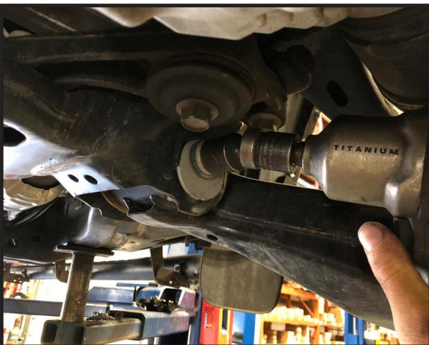
8. Remove the bolts that attach the sway bar endlinks to the lower control arms
