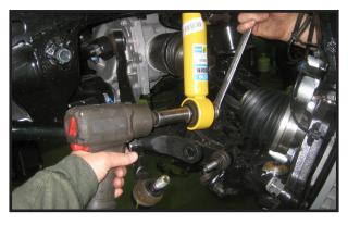
13. Move back to the (3) 3/8" upper nuts and torque to 32 ft 16. At this time repeat steps #2 - #15 on the passenger side
