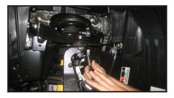
Using a hammer, carefully strike the steering knuckle to seperate the upper ball joint from it. Take special care not to damage the rubber boot on the ball joint.
