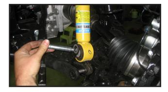
Remove the strut assembly from the vehicle and place on work bench.
