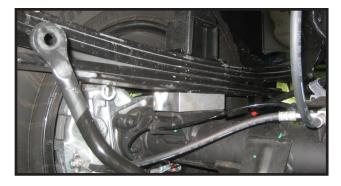
24. Locate and install the new rear Ubolts with the new nuts and washers. Torque to 105 ft lbs.
