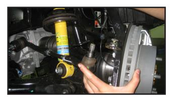
6. Disconnect the sway bar endlink from the swaybar.
