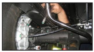
23. Install the new lift block between the axle perch and bottom of the leaf spring pack. SPECIAL NOTE: the lift block has a slight taper and needs to be installed so the thicker side is towards the rear of the vehicle.
