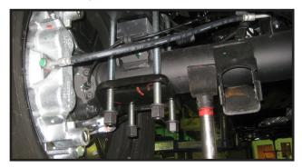
Repeat steps #18 - 24 on the Passenger side and install new rear shocks.
