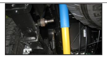
21.Remove the rear shocks completely and save the mounting hardware.
