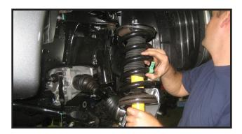
10. Locate one of the 52008-01 strut spacers and also locate (3) OE nuts for the top of the strut. Install the new spacer on top of the strut using the OE nuts and torque to 45 ft lbs.
