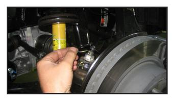
5. Using the same method as the upper ball joint, seperate the outer tierod end from the steering knuckle.
