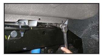
22. With the axle being supported from underneath, remove the OE ubolts and lower the axle enough to install the new lift block.
