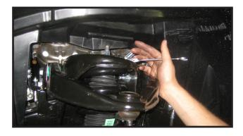
8. Move the the lower strut mounting bolt and remove the hardware. Save hardware for re-installation. Once this bolt is removed, take extra care to not let the suspension drop so far that it binds up the axle and pulls hard on the brake lines.
