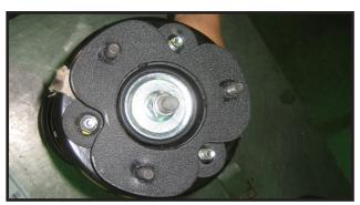
11. Locate (3) 38NLN nuts and (3) 516WA washers from hardware bag D2PNB. Install the strut back into the vehicle and loosley start the new 3/8" nuts on the top.
