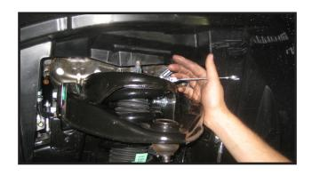
8. Move the the lower strut mounting bolt and remove the hardware. Save hardware for re-installation. Once this bolt is removed, take extra care to not let the suspension drop so far that it binds up the axle and pulls hard on the brake lines.
