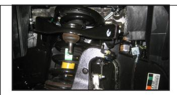
4. Remove the cotter pin from the outer tie rod end and save the cotter pin.
