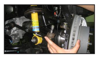
6. Disconnect the sway bar endlink from the swaybar.
