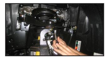
3. Using a hammer, carefully strike the steering knuckle to seperate the upper ball joint from it. Take special care not to damage the rubber boot on the ball joint.
