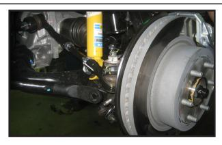
of the vehicle. Once complete re-install the swaybar endlinks to the sway bar and torque to 45 ft lbs.
