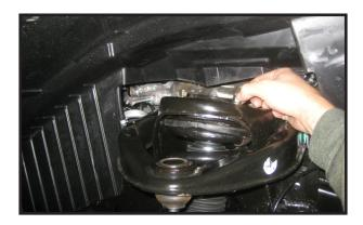
12. Re-install the OE lower strut hardware to the lower control arm and torque to 120 ft lbs.
