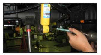
22. With the axle being supported from underneath, remove the OE ubolts and lower the axle enough to install the new 25. Re-attach the sway bar end link to the sway bar lift block.
