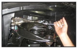
14. Re-attach the upper ball joint to the steering knuckle using the OE nut and Cotter pin. Torque to 75 ft lbs.
