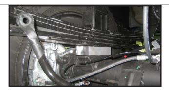
21. Remove the lower shock mounting bolts and save them. 24. Locate and install the new rear Ubolts with the new nuts and washers. Torque to 105 ft lbs.
