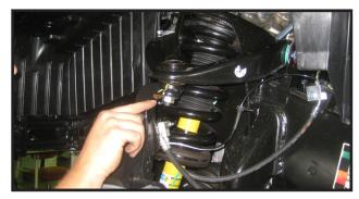
15. Re-install the tie rod end to the steering knuckle using the OE nut and cotter pin. Torque to 75 ft lbs.
