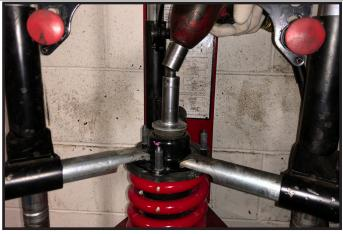
15. Remove the strut assembly from the strut compressor and take it back over to the vehicle. Install the strut back into the original location and use OE nuts to loosely hold the strut in place.
