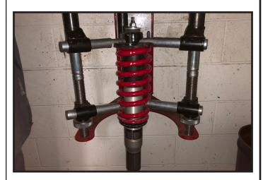
Carefully compress the strut until the upper hardware can be removed. Remove the nut and hardware and save for re-assembly.
