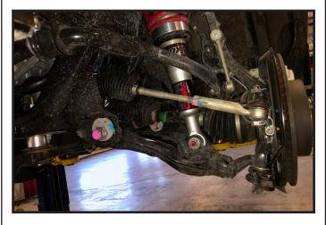
17. Raise the lower control arm up even more until you can re-install the 2 lower ball joint bracket bolts to the steering knuckle. Torque to 160 ft lbs.
