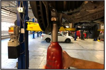
6. Loosen, but do not remove the lower control arm cam adjusting bolts.
