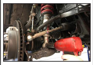
trol arm ball joint piece to the steering knuckle.
