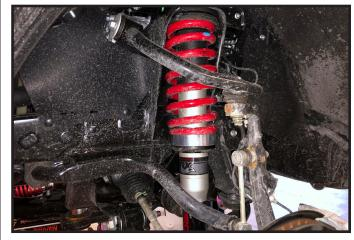
16. Raise the lower control arm back up until you can install the OE lower mounting bolt and hardware. Leave this loose for now.
