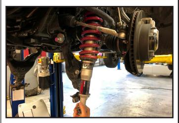
Tuff Country EZ-Ride Suspension recommends a wall mounted strut compressor be used when performing the steps that talk about installing the spacer into the strut. If you do not have a wall mounted strut compressor, please have these steps performed by your local Toyota Dealership
