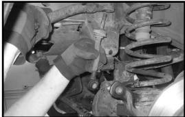
4. Working on the driver side, remove the brake line bracket from OE location. Save the hardware. Repeat procedure on
