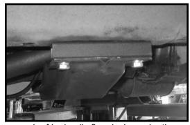
31. Place a pair of hydraulic floor jacks under the rear differential. Place one on the driver and passenger side. Carefully raise up on both floor jacks until they come into contact with the rear differential.
