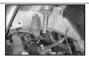
9. Locate the new coil springs. Working on the driver side, install the new coil spring into the OE location. Repeat procedure on the passenger side.
