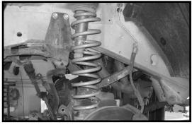
10. Carefully raise up on both hydraulic floor jacks until the newly installed coil springs seat properly into the lower coil spring pockets. Locate and install the OE coil spring clip using the OE hardware on the driver side. Make sure to use loctite and torque to **12 ft lbs.** Repeat procedure on the passenger side.
