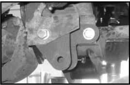
bracket to the OE pocket and add some loctite and torque to shock into the OE location using the lower mounting hard-28 ft lbs.
