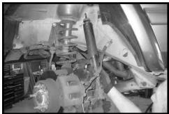
Working on the driver side, remove the sway bar endlink from the sway bar and axle location. Save the hardware and endlink. Repeat procedure on the passenger side
