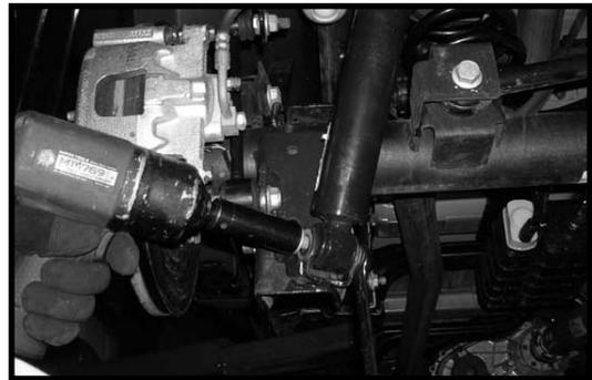
30. Locate the stock end link mounting hardware. Working on the driver side, install the stock rear sway bar end link into the stock lower mounting location and secure using the stock hardware. Make sure to use thread locker or loctite and torque to **45 ft lbs**. Repeat procedure on the passenger side.
