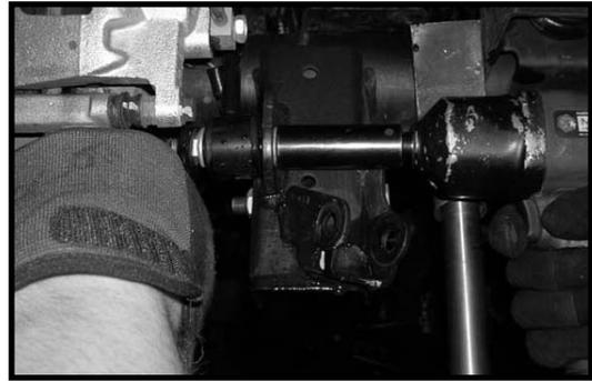
17. Working on the driver side, remove the stock bolt holding the stock brake line bracket to the side of the stock frame rail. Save the stock bolt for later re-installation. Repeat procedure on the passenger side.
