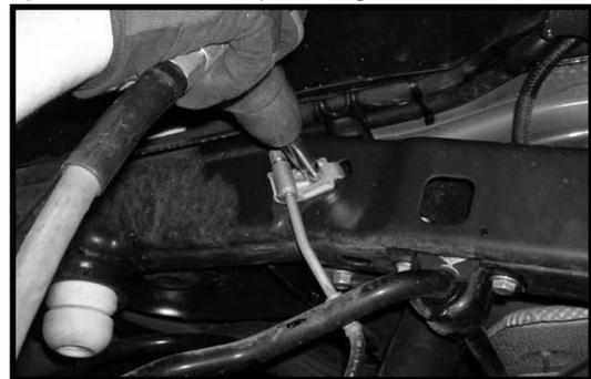
18. Working on the driver side, carefully remove the stock ABS line clip from the bottom side of the stock frame rail. **Special note: Take special care not to damage the ABS line clip during removal. This will need to be re-installed back into the same hole at a later step.** Repeat procedure on the passenger side.
