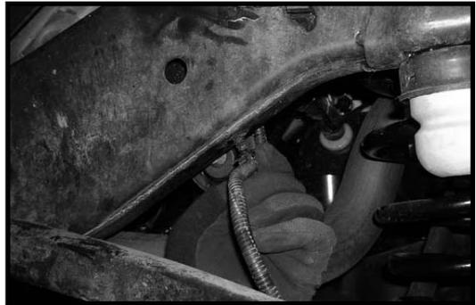
22. Locate the stock brake line hardware. Working on the driver side, re-install the stock brake line bracket to the side of the stock frame rail using the stock hardware. Repeat procedure on the passenger side.
