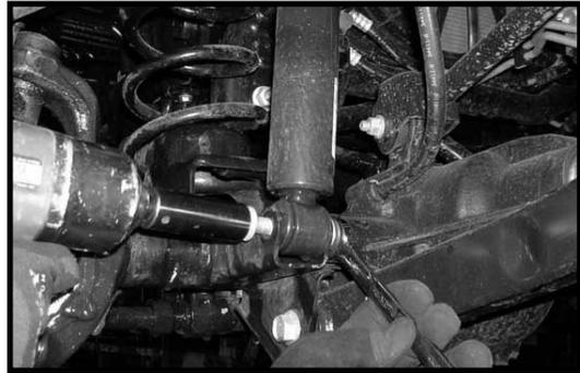
5. Carefully lower down on both hydraulic floor jacks until the front coil springs can be removed. Working on the driver side, remove the stock coil spring. Set aside for later re-installation. Repeat procedure on the passenger side. **Special note: Make sure to keep the driver and passenger side coil springs separate from each other. We need to make sure that the driver side coil spring gets installed back into the vehicle on the driver side and the same with the passenger side.**
