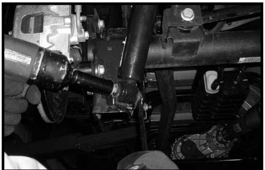
24. Locate the stock end link mounting hardware. Working on the driver side, install the stock rear sway bar end link into the stock lower mounting location and secure using the stock hardware. Make sure to use thread locker or loctite and torque to **45 ft lbs**. Repeat procedure on the passenger side
