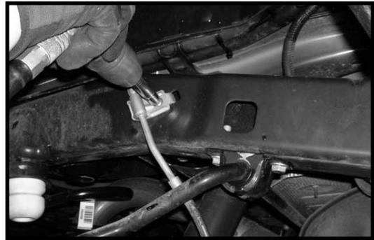
29. Locate the stock lower shock mounting hardware. Working on the driver side, install the stock shock into the stock lower mounting location and secure using the stock hardware. Make sure to use thread locker or loctite and torque to **65 ft lbs**. Repeat procedure on the passenger side.
