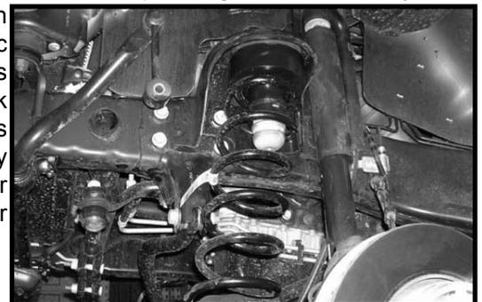
8. Locate the stock lower shock mounting hardware. Working on the driver side, install the stock shock into the stock lower mounting location and secure using the stock hardware. Make sure to use thread locker or loctite and torque to **65 ft lbs**. Repeat procedure on the passenger side.
