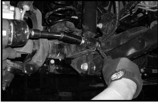
9. Locate the stock front end link mounting hardware. Working on the driver side, install the stock front sway bar end link into the stock lower mounting location and secure using the stock hardware. Make sure to use thread locker or loctite and torque to **45 ft lbs**. Repeat procedure on the passenger side.
