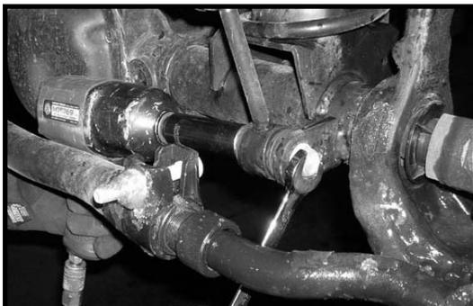
4. Working on the driver side, remove the stock mounting hardware that connects the stock shock into the stock lower mount. Save the stock hardware for later re-installation. Repeat procedure on the passenger side. **Special note: There is no need to remove the shock completely from the vehicle. Keep the stock shock mounted to**
