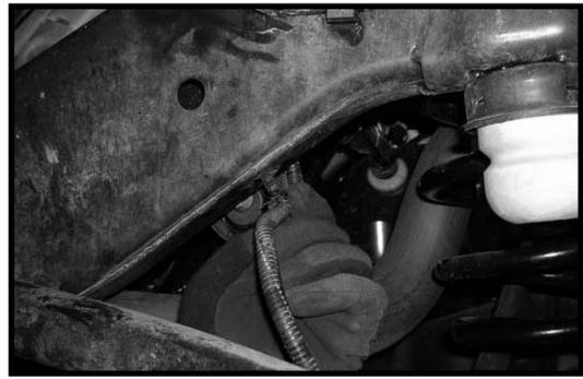
28. Locate the stock brake line hardware. Working on the driver side, re-install the stock brake line bracket to the side of the stock frame rail using the stock hardware. Repeat procedure on the passenger side.
