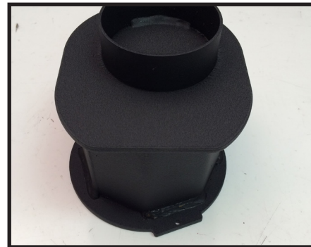
Part # 35130-03 / Qty. 1 driver side front coil spacer
