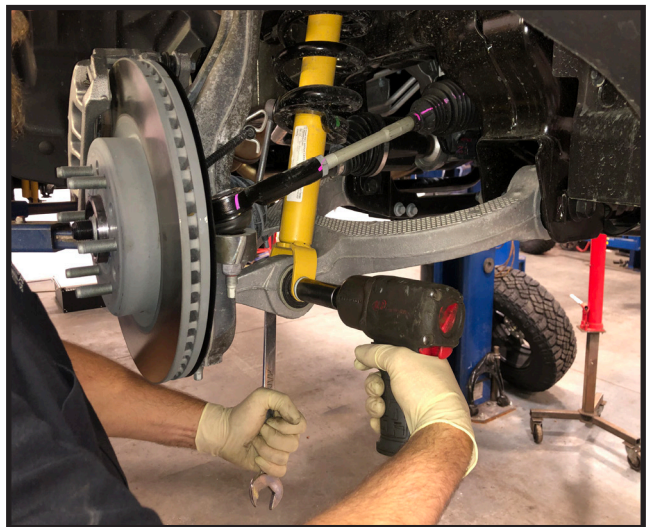
13. Loosen but do not remove the lower strut mounting bolt and hardware.
