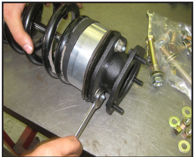
24. Locate a new upper strut spacer part #33505-01, Install it on top of the OE strut and secure using the OE hardware.
