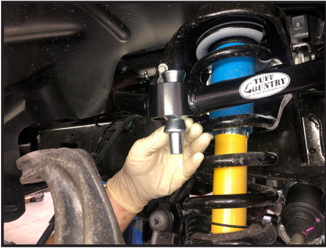
12. Remove 2 of the 3 upper strut mount nuts and loosen the 3rd one.
