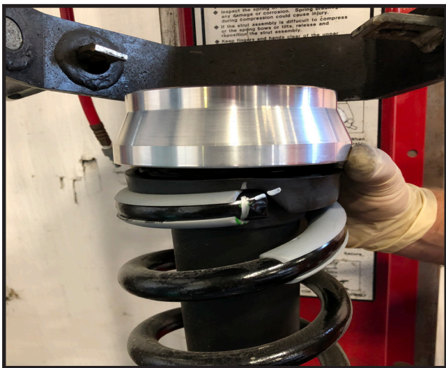
21. Re- install the top strut plate making sure to line up your
