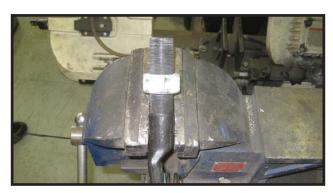
Now working on the drag link portion that is still connected to the vehicle, carefully cut the half round locking portion off of this end.
