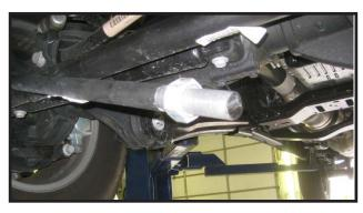
10. Re-connect the drag link and tierod end using the adjuster sleeve. Install the rod end into the new pitman arm. **Special note:** the new pitman arm is tappered opposite from the **OE pitman arm, so the rod end will now be installed from the bottom.** Secure the rod end to the pitman arm using the OE hardware and torque to **85 ft lbs.** Make sure to re-tighten the 2 large jam nuts on the adjuster sleeve.
