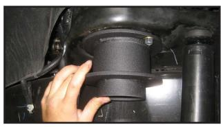
18. Locate the OE coil spring rubber isolator. Working on the driver side, install the rubber isolator to the newly installed coil spring spacer. Special note: Make sure that the nipple of the isolator fits properly into the hole on the lower ring of the coil spacer. Repeat procedure on the passenger side.
