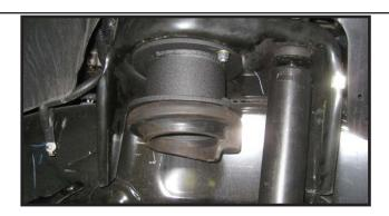
19. Locate the OE coil springs. Working on the driver side, install the coil spring back into the vehicle. Carefully raise up on the hydraulic floor jack until the coil spring seats properly into the new coil spacer. Repeat on the passenger side.
