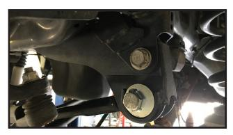
16. Carefully lower down on both hydraulic floor jacks at the same time allowing enough room for the coil springs to be removed. Working on the driver side, remove the coil spring and set aside. Repeat procedure on the passenger side. Special note: take special care not to over extend any brake lines or hoses.
