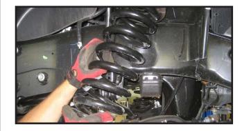
17. Locate the new coil spring spacers, Also, locate (2) 3/8" x 1" bolts, (4) 5/16" flat washers, and (2) 3/8" unitorque nuts from hardware bag 33119NB1. Working on the driver side,
