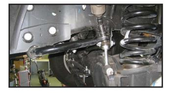
5. Working on the driver side, remove the nut that connects the draglink tierod end to the pitman arm, save the nut. Using a hammer, carefully strike the pitman arm to break the taper of the tie rod end. Special Note: Take extra care not to rip or tear the draglink tie rod end boot.
