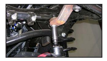
6. Next, remove the nut and lock washer from the steering gear box. Save the hardware. Using a pitman arm puller, carefully remove the pitman arm from the steering gear, the stock pitman arm may be discarded.
