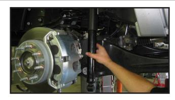
4. Working on the driver side, remove the sway bar end link from the sway bar. Save the hardware. Repeat procedure on the passenger side.
