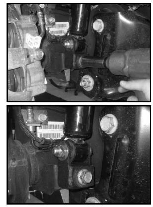
12. Working on the driver side, install the sway bar back to the sway bar end link and secure using the OE hardware. Make sure to use loctite and torque to **40 ft lbs.** Repeat procedure on the passenger side.
