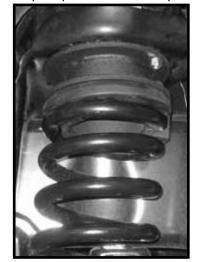
11. Working on the driver side, install the modified shock into the upper and lower location using the OE hardware. Make sure to use loctite and torque the lower mounting hardware to **85 ft lbs.** and the upper mounting hardware to **22 ft lbs.** Move back to the new 9/16" hardware and add some loctite and torque to **85 ft lbs.** Repeat procedure on the passenger side.
