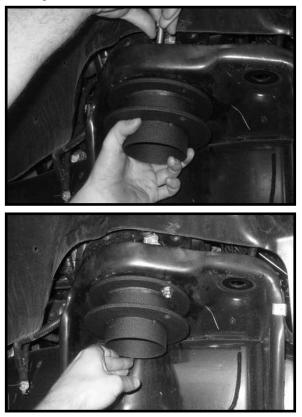
9. Locate the OE upper coil spring isolator and coil springs. Working on the driver side, install the isolator to the top of the coil spring and install the coil spring back into the vehicle. Carefully raise up on the hydraulic floor jack until the coil spring and isolator seat properly into the newly installed coil spring spacer. Repeat procedure on the passenger side.
