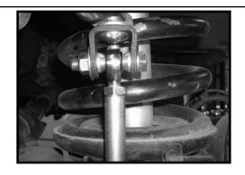
Using a 9/16" drill bit, carefully drill out the lower sway bar end link hole.
