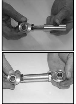
8. Locate (1) 1/2" x 2 1/2" bolt, (2) 7/16" flat washers, (1) 1/2" unitorque nut and (2) S10194 conned sleeves from hard ware bag 30927NB and 30927SL. Install the new al thread sleeve and hiem joints to the upper bracket using the new hardware and conned washer. Make sure to follow the photo's to properly install the conned sleeves. Make sure to use loctite and torque to **70 ft lbs**.
