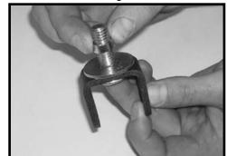
end link and all hardware may be discarded. Repeat proce-from hardware bag 30927NB. Install the new bracket to the stock sway bar and secure using the new hardware. Make sure to use loctite and torgue to 70 ft lbs. Special note:
