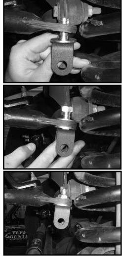
Locate (1) S10195 all thread sleeve and (2) S10116 hiem joints from hardware bag 30927NB and 30927SL. Install the new hiem joints into each end of the new all thread sleeve.
