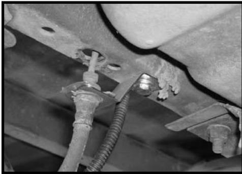
19. Locate the stock sway bar end link hardware. Working on the driver side, secure the stock sway bar end link to the stock sway bar using the stock hardware. Make sure to add some thread locker or loctite and torque to **32 ft lbs**. Repeat procedure on the passenger side.
