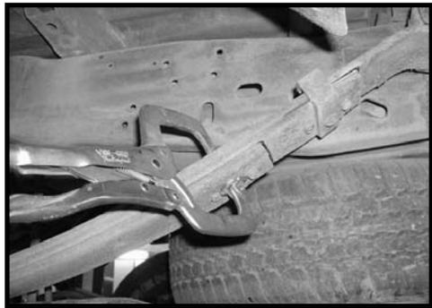
8. Carefully remove the stock centering bolt from the stock location and discard. **Special note: Once the stock centering bolt has been removed, the stock over load will fall out. Save the stock over load.** Repeat procedure on the passenger side.
