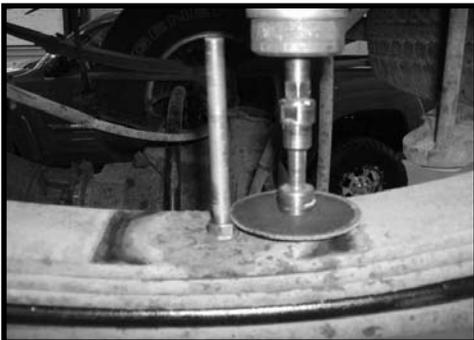
11. Locate the new blocks. Working on the driver side, install the new block into the stock location. **Special note: If the new block that you are installing has a taper to it, make sure to install the smaller end of the block towards the front of the vehicle.** Repeat procedure on the passenger side. Carefully raise up on both hydraulic floor jacks that are holding the rear axle until the new blocks make contact with the stock springs.
