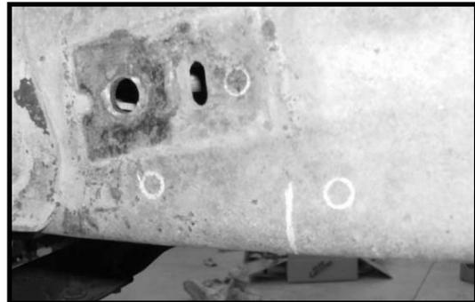
Repeat steps # 19 - # 23 excluding # 20 to make sure that the holes are in the correct location before drilling into the frame rail. This is an important step, so we want to make sure that the extended radius arm relocation bracket is in the correct location so when the extended radius arm is attached to it, the twin eye beam axle is not sitting too far forward or too far rearward.
