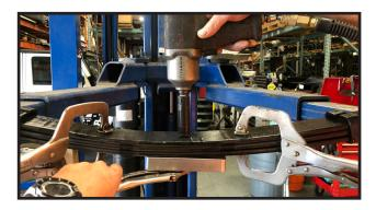
34. Raise the rear axle up to the block and spring. Locate part # 5U-247s and part # 916nw. install new ubolts and hardware. Dont tighten at this time. Repeat steps 28-34 on passenger side. Once passenger side is completed, Tighten ubolts to 90 ft-lbs.
