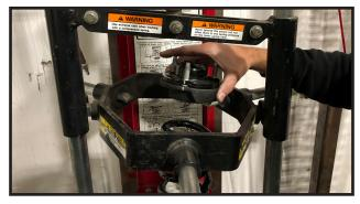
13. Locate part # S10305 washer and install onto the shock stud.
