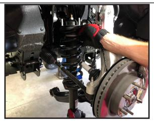
8. Using a hammer and a vice. Remove the two studs on the lower strut mount. Thread the nut on the stud to prevent damage to the stud. Save Hardware.
