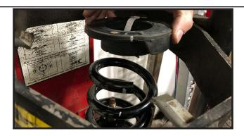
17. Locate part # 23105-01 strut top hat. Install top hat on top of the rubber isolator. Line up one of the studs on the top hat to your mark on the isolater.
