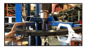
if your not replacing them remove the lower shock bolt only. bag. Using the center pin from cb38 hardware bag, bolt 23105-02 to the bottom of the leaf spring. Tighten to 35 ft-lbs.
