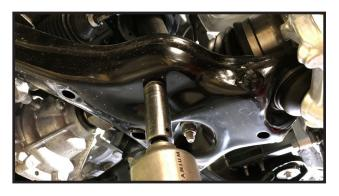
3. Remove the driver and passenger side lower conrol arm cam bolt nuts. Save hardware.
