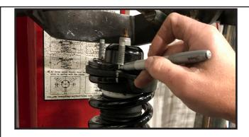
11. Mark the coil and lower coil spring seat
