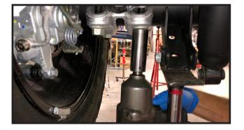
31. Lower axle down from leaf spring. There is a spacer plate on the bottom of the spring. Make sure that goes back in the same spot.
