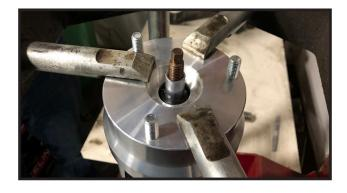
19. Locate part # M22706 poly bushing, S10305 washer and M12NLN 12 MM nylock nut. install them onto the shock stud. Tighten untill the nut bottoms out.
