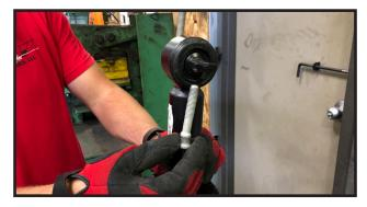
Using a wall mount strut compressor, Place strut in strut compresor.
