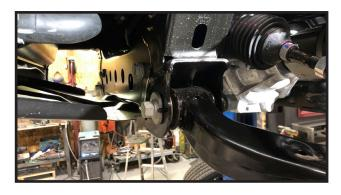
23. Tighten the lower strut studs untill they'er pulled in all the way in flush. Back nut off one turn, Then Tighten to 90f t lbs.
