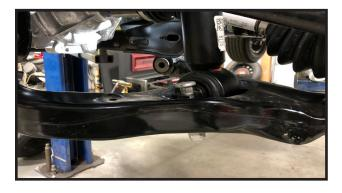
22. Locate OEM lower control arm cam bolt hardware. Using a jack, Raise lower control arms into frame mounts. Install Carefully lower the vehicle back down to the ground and front and rear cam bolts and nuts into lower control arm remove the jacks. mounts. Leave loose.
