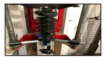
10. Mark the coil and rubber isolator on the top of the strut.
