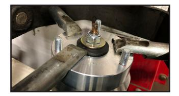
20. Locate part # 38FLN 3/8 flange nut. Re install strut into top strut mount, Using 3 three of the 38FLN. leave loose for now.
