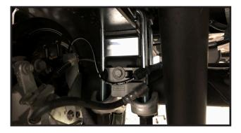
35. Re install lower shock mount. If replacing shocks. install new shocks.
