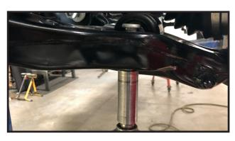
21.On driver and passenger, Raise the lower control arm 24. Working on the top strut mounts. Tighten the three nuts
