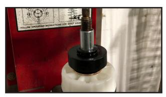
16. Locate the strut rubber coil isolater and install it onto the top of the coil, Make sure to line your marks up.
