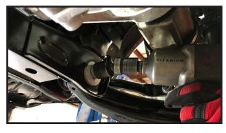
Remove the driver and passenger side cam bolts. Save hardware.
