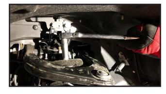
7. Mark which strut is driver side and which is passenger side.
