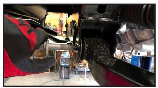
5. Lower the lower control arm out of the mounting pocket on the driver and passenger side.
